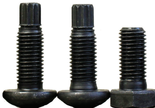
Fig. 5. Three \frac{7}{8} -in.-9 \times 2-in. bolts manufactured by three different manufacturers.
