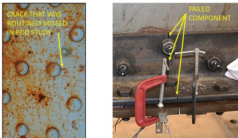
Fig. 1. Photographs of two different cracks in built-up members contrasting the differences in cracks that need to be detected in a traditional FCM inspection vs. those associated with an IRM.
