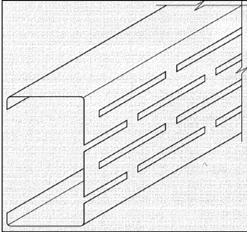
Figure 2-7: Channel Section with Slotted Web
