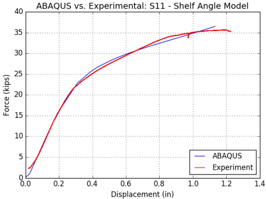
Figure 6-25 Assembly S11 – Force-Displacement, ABAQUS vs. Experimental
