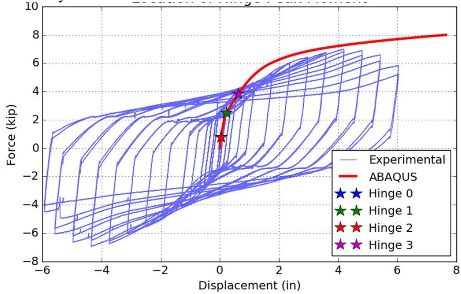
Figure 7-31: Assembly C13 – Force-Displacement, ABAQUS vs. Experimental
