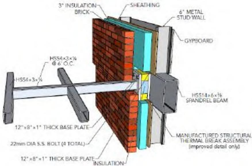
Figure 1-6: Canopy beam typical details (from D'Aloisio 2012)
