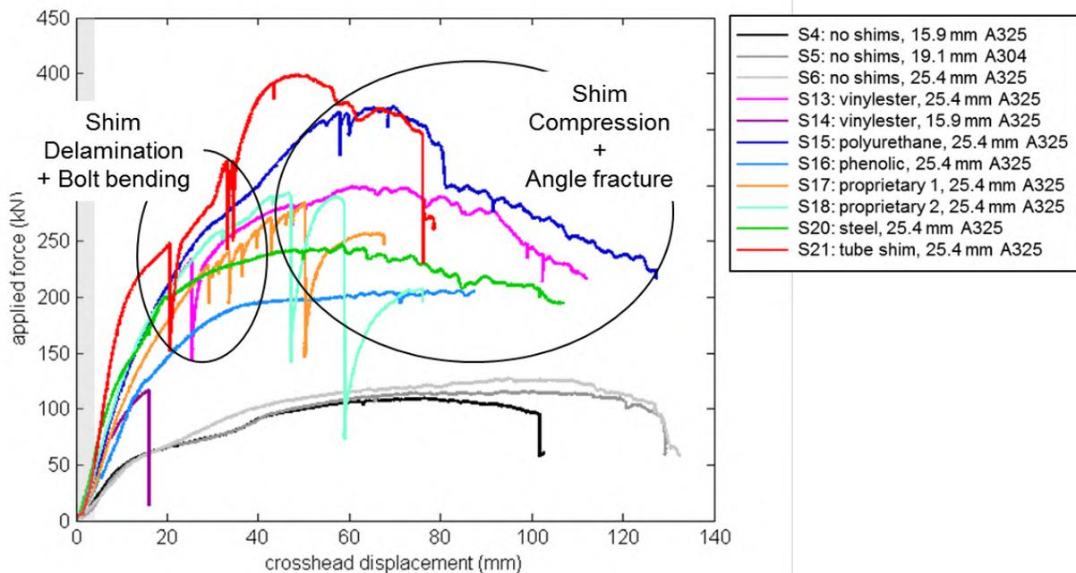
Figure 6-7: Force-displacement results for climate zone 7 specimens, indicating progression of failure for FRP shims.
