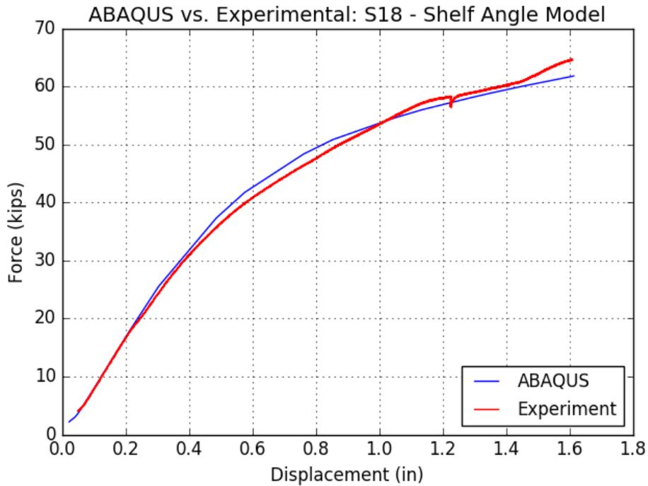
Figure 6-39 Assembly S18 – Force-Displacement, ABAQUS vs. Experimental
