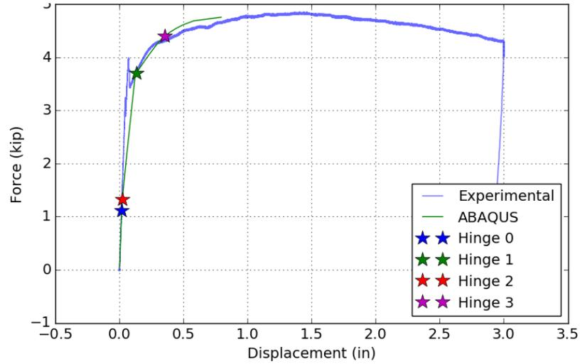
Figure 7-35: Assembly R1 – Force-Displacement, ABAQUS vs. Experimental
