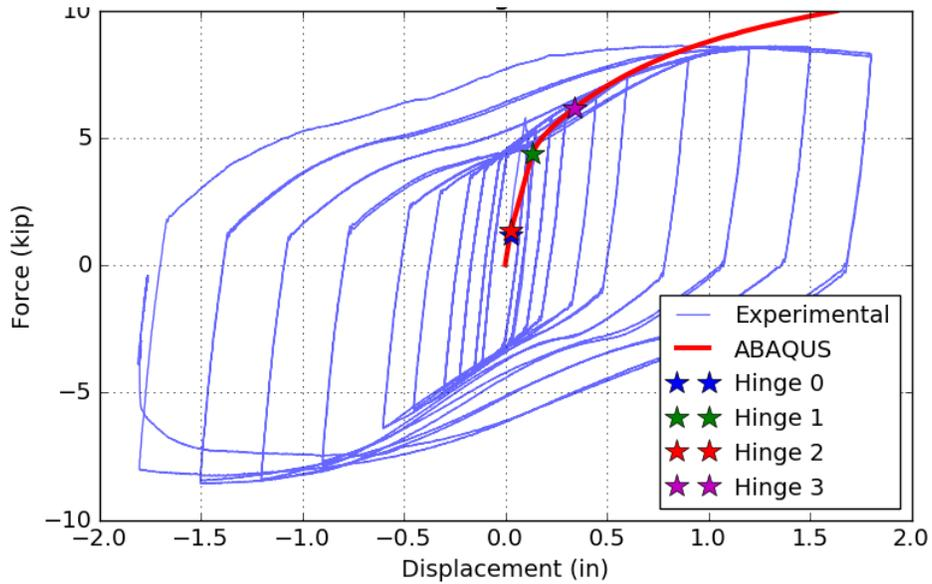
Figure 7-45: Assembly R14 – Force-Displacement, ABAQUS vs. Experimental
