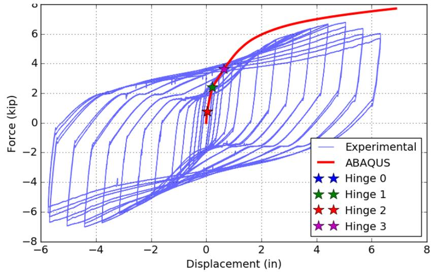
Figure 7-29: Assembly C8 – Force-Displacement, ABAQUS vs. Experimental
