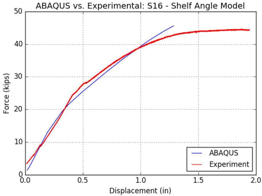
Figure 6-35 Assembly S16 – Force-Displacement, ABAQUS vs. Experimental
