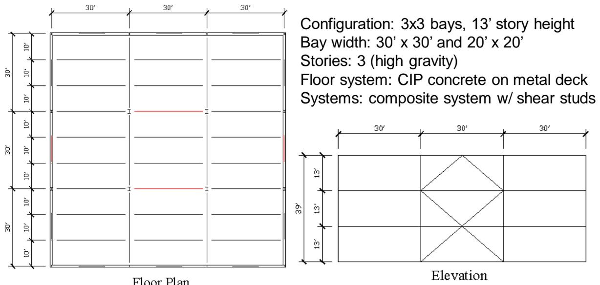
Figure 1-1: Archetypal building design: floor plan view and elevation. The location of the SCBFs is shown in red. Composite system refers to concrete floor slab systems.
