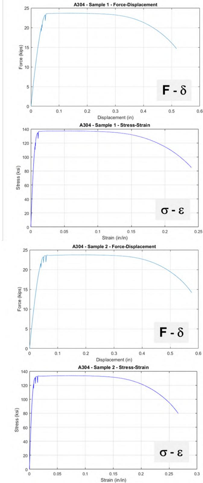
Figure A-64: Force-displacement and stress-strain relationships for A304-SH1 base metal bolt testing
