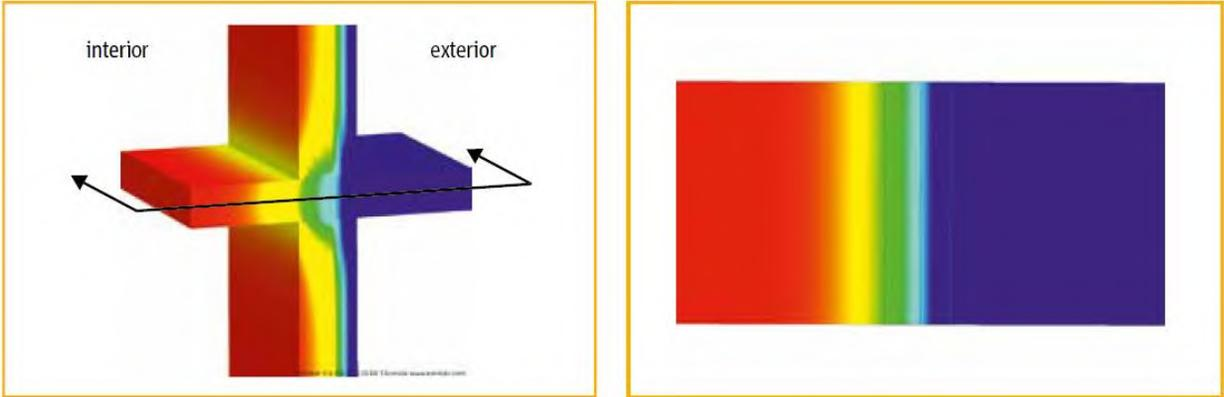
Figure 2-12: Linear thermal bridge in a balcony connection (Schoeck Ltd 2015)
