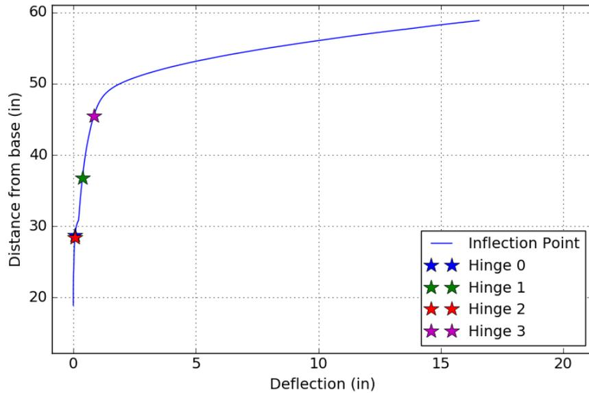
Figure 7-28: Assembly C7 –Inflection Height
