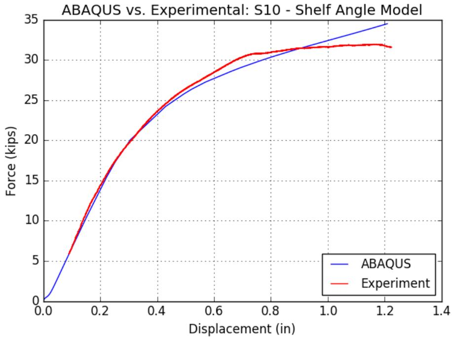
Figure 6-23 Assembly S10 – Force-Displacement, ABAQUS vs. Experimental
