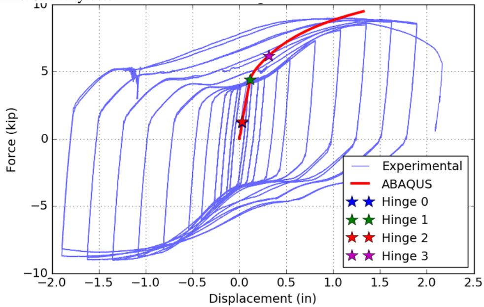
Figure 7-41 Assembly R8 – Force-Displacement, ABAQUS vs. Experimental
