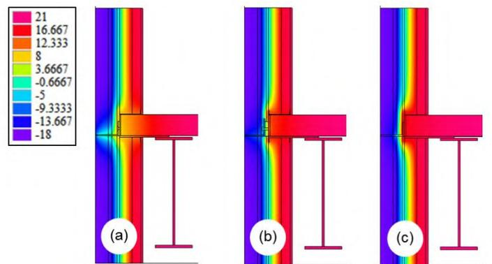
Figure 3-22: Thermal modeling of slab-supported shelf angles in climate zone 1 with a 2.5" cavity width 2D results and comparisons: a) Unmitigated, b) Vinylester shim ( $\Delta\psi=81\%$ ), c) FRP angle ( $\Delta\psi=92\%$ )
