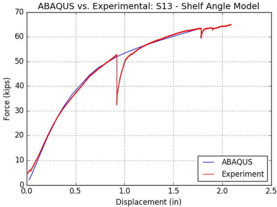
Figure 6-29 Assembly S13 – Force-Displacement, ABAQUS vs. Experimental
