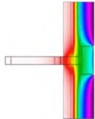
Figure 2-32: Thermal Gradient, Unmitigated (D'Aloisio, et al. 2012)
