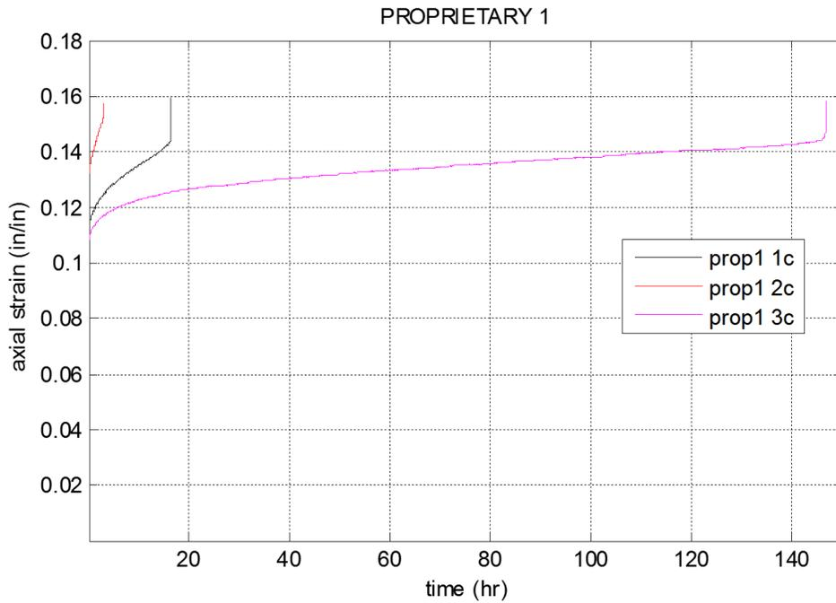
Figure 4-18: Strain versus time for proprietary 1 creep specimens
