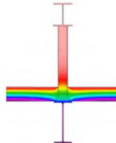
Figure 2-18: Mitigated roof post (D'Aloisio, et al. 2012)
