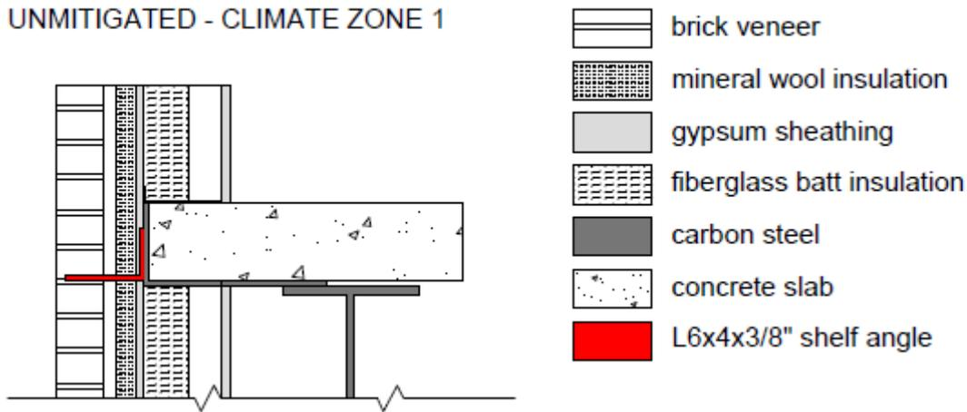
Figure 1-4: Unmitigated slab-supported shelf angle detail, climate zone 1
