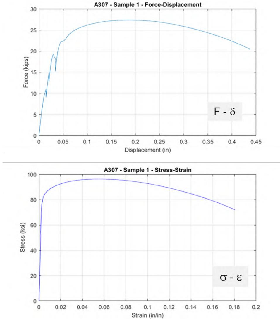
Figure A-65: Force-displacement and stress-strain relationships for A307 base metal bolt testing. Results across all base metal bolt testing are shown in Table A-35 below. Modulus of elasticity, static yield stress, dynamic yield stress, and ultimate stress are reported.
