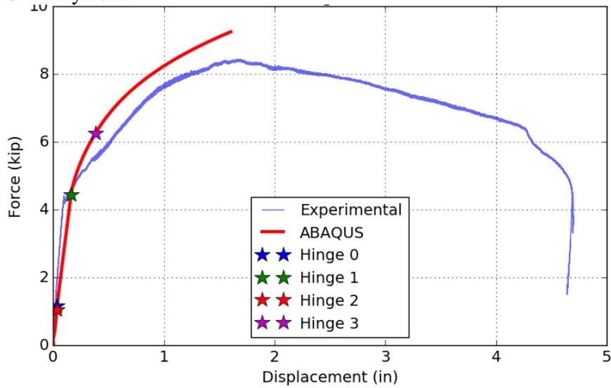
Figure 7-37: Assembly R2 – Force-Displacement, ABAQUS vs. Experimental
