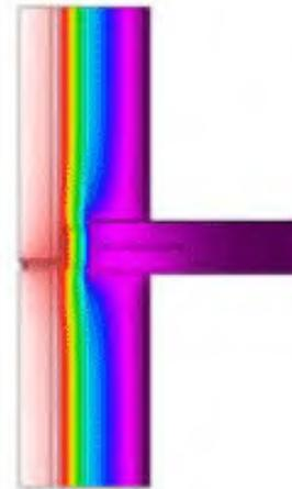
Figure 2-26: Thermal Gradient, Mitigated (D'Aloisio, et al. 2012)
