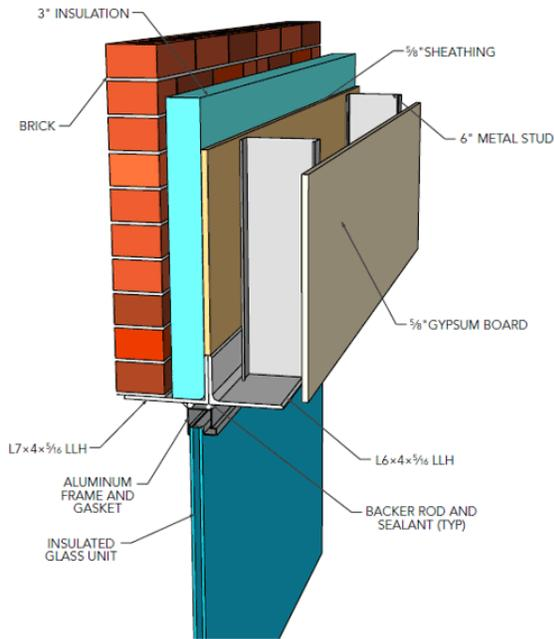
Figure 2-27: Masonry Lintel, Unmitigated (D'Aloisio, et al. 2012)
