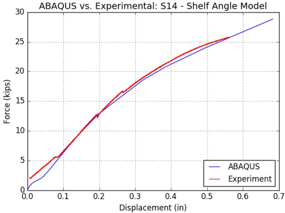
Figure 6-31 Assembly S14 – Force-Displacement, ABAQUS vs. Experimental
