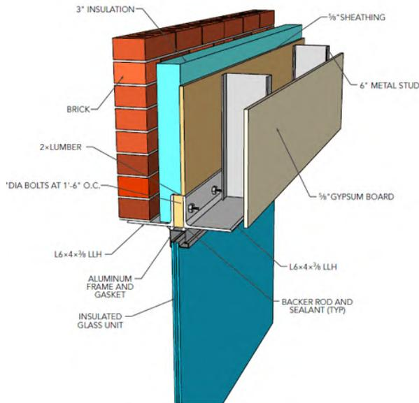
Figure 2-29: Masonry Lintel, Mitigated (D'Aloisio, et al. 2012)
