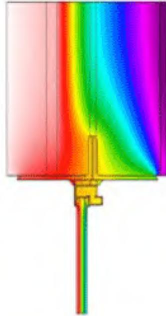
Figure 2-28: Thermal Gradient, Unmitigated (D'Aloisio, et al. 2012)
