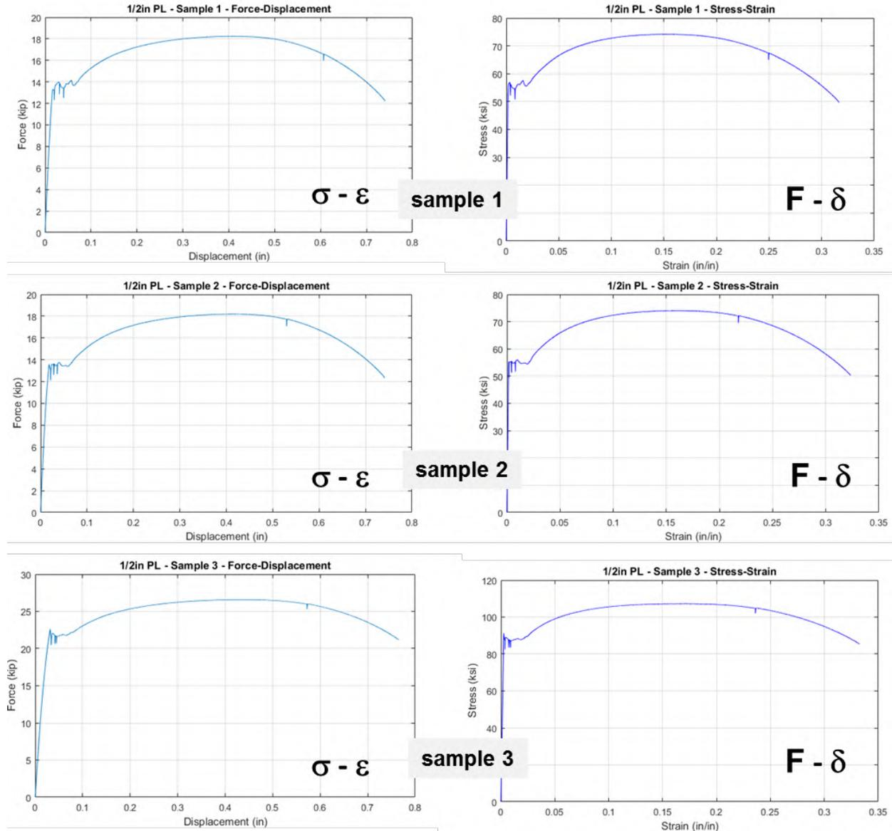
Figure A-59: Force-displacement and stress-strain results for base metal tensile tests of 1/2" base plate specimens
