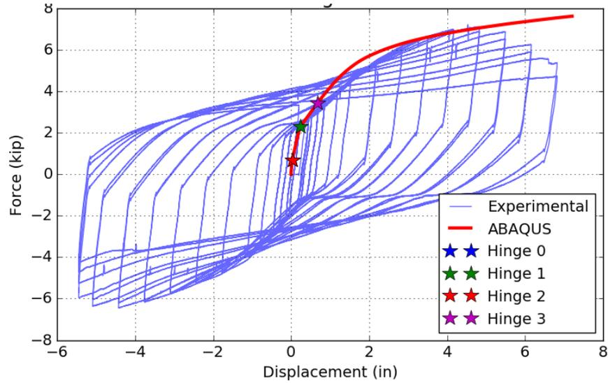
Figure 7-33: Assembly C15 – Force-Displacement, ABAQUS vs. Experimental
