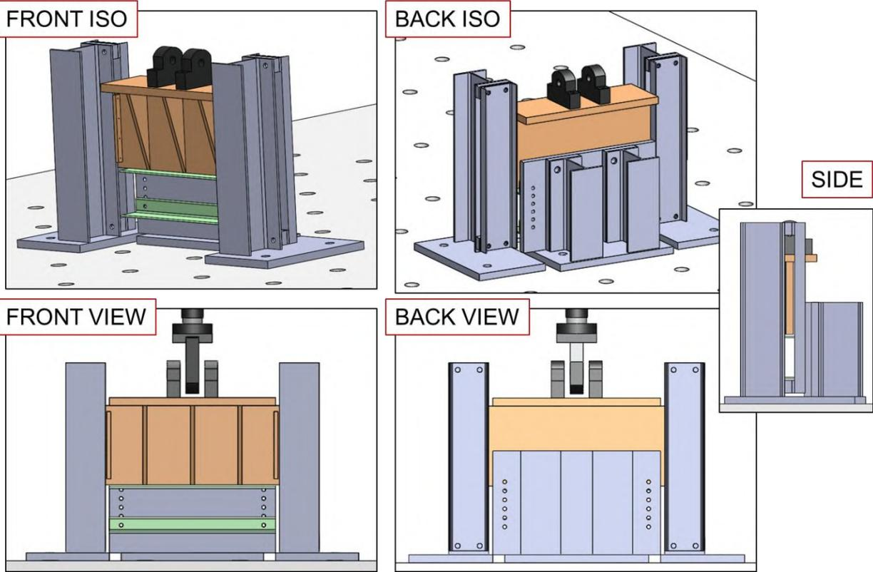
Figure 6-2: Detail views of shelf angle test rig
