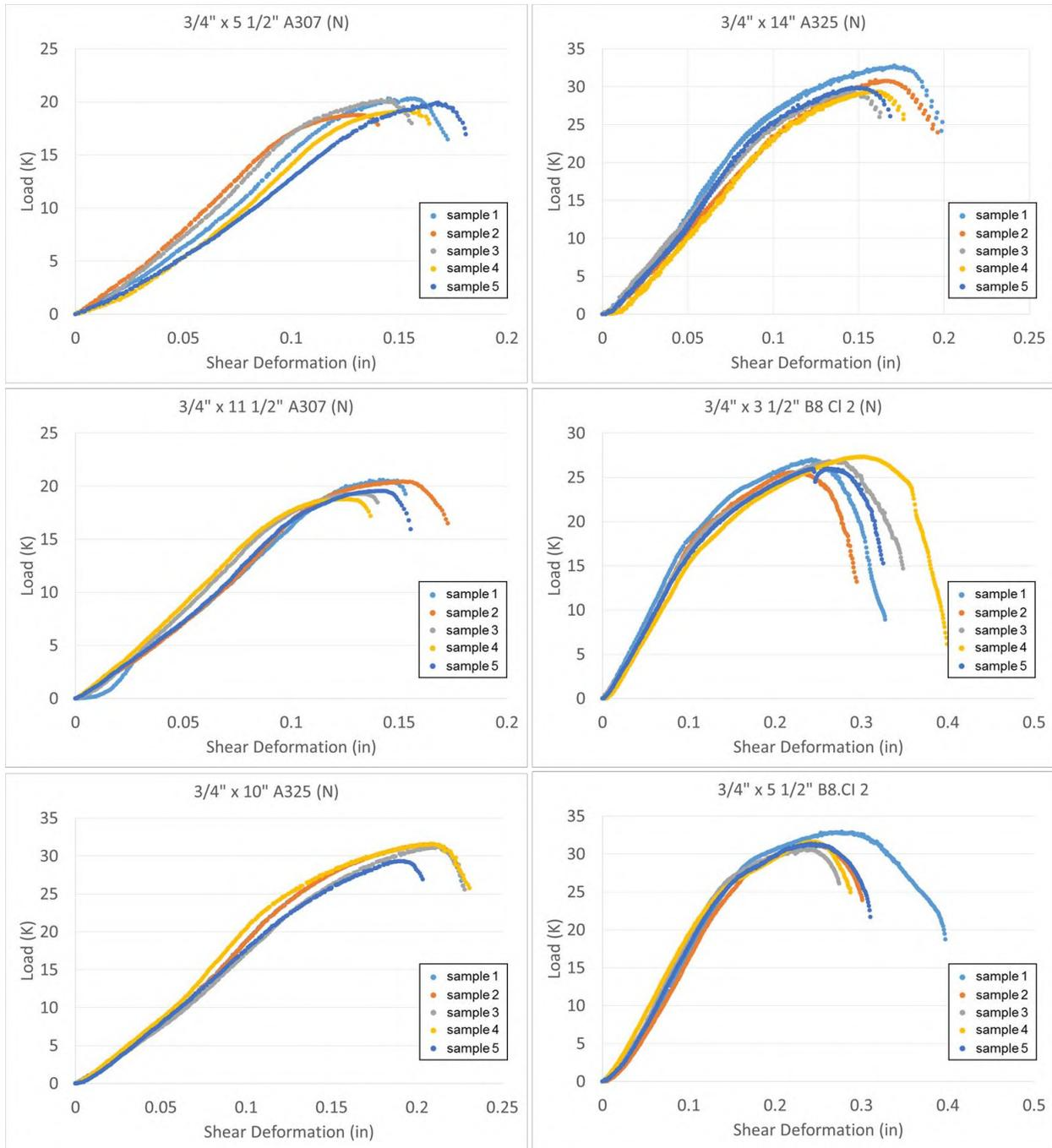
Figure A-74: Force-displacement results for 3/4" diameter bolt and rod shear testing
