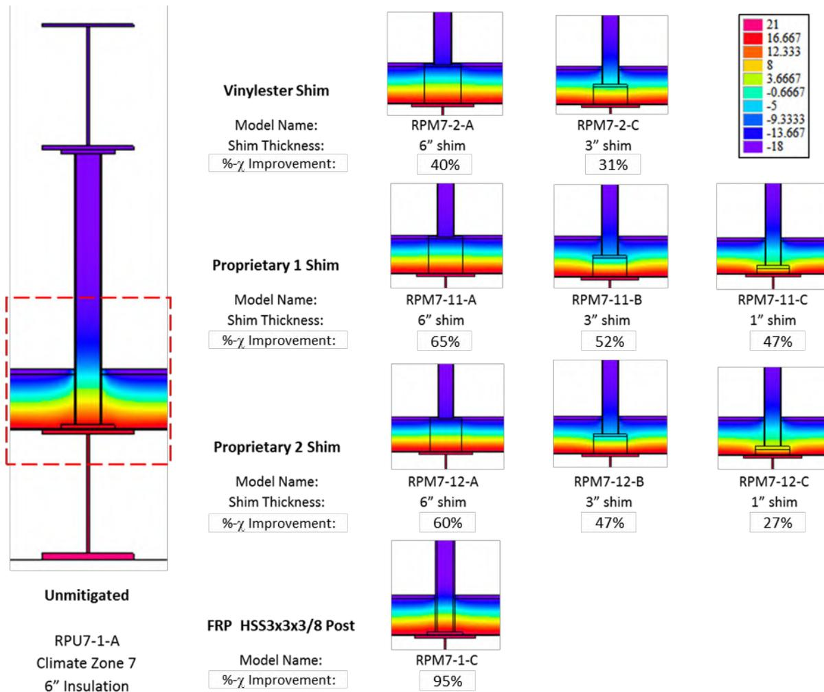
Figure 3-16: Thermal modeling of roof posts in climate zone 7 (6" insulation thickness) 2D results and comparisons
