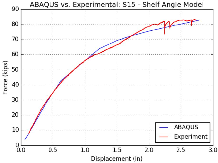
Figure 6-33 Assembly S15 – Force-Displacement, ABAQUS vs. Experimental
