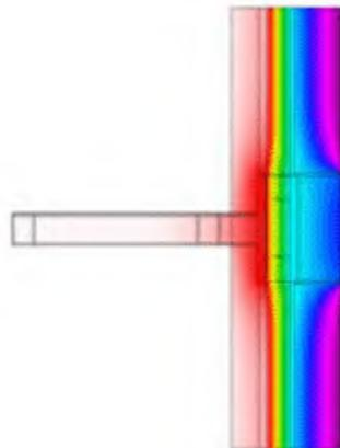
Figure 2-33: Thermal Gradient, Mitigated (D'Aloisio, et al. 2012)
