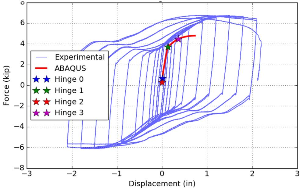
Figure 7-39: Assembly R7 – Force-Displacement, ABAQUS vs. Experimental
