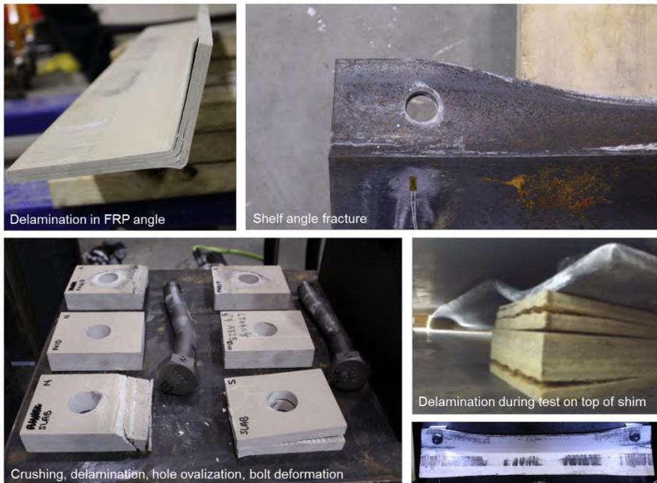
Figure 6-10: Typical failure modes observed during testing
