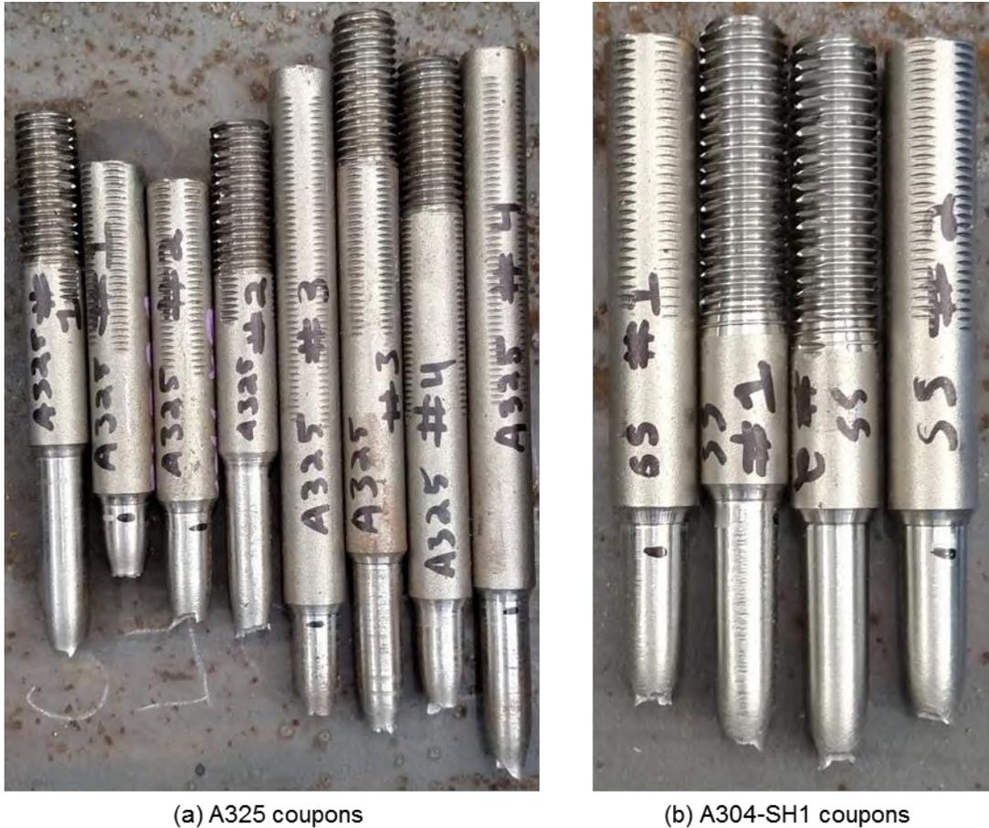
Figure A-61: Photographs of A325 and A304-SH1 specimens after testing
