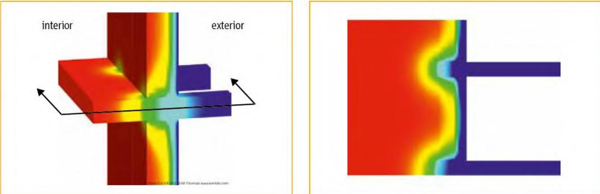
Figure 2-13: Point thermal bridge in a balcony connection (Schoeck Ltd 2015)
