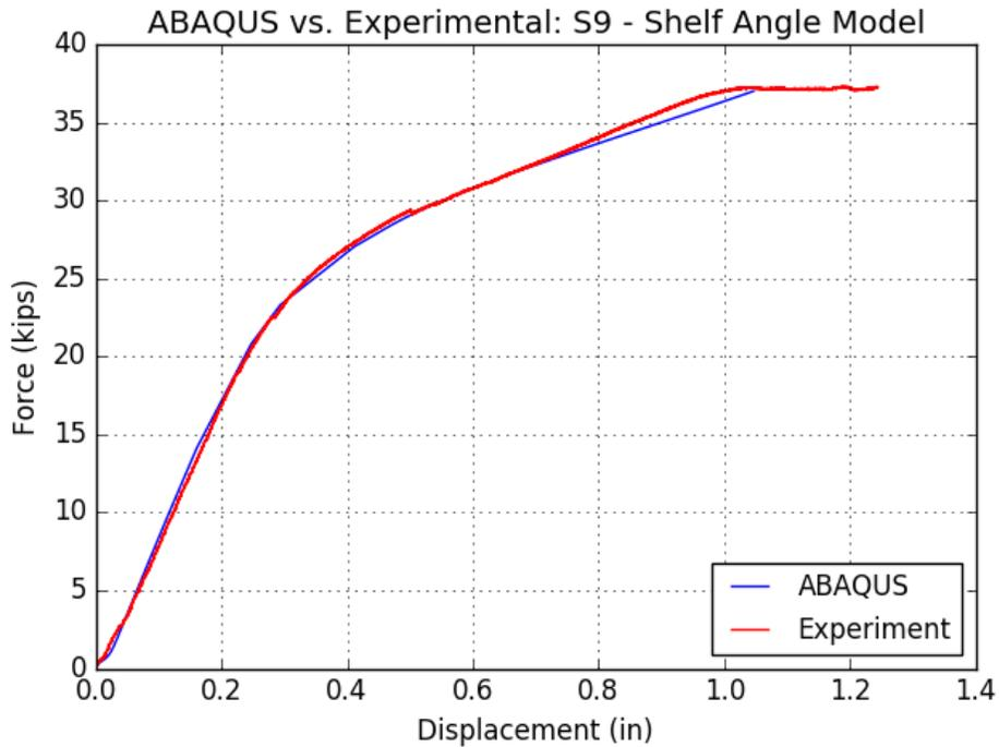
Figure 6-21 Assembly S9 – Force-Displacement, ABAQUS vs. Experimental
