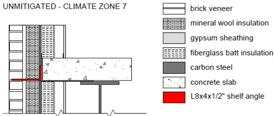
Figure 1-5: Unmitigated slab-supported shelf angle detail, climate zone 7
