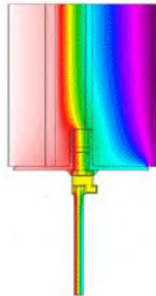
Figure 2-30: Thermal Gradient, Mitigated (D'Aloisio, et al. 2012)
