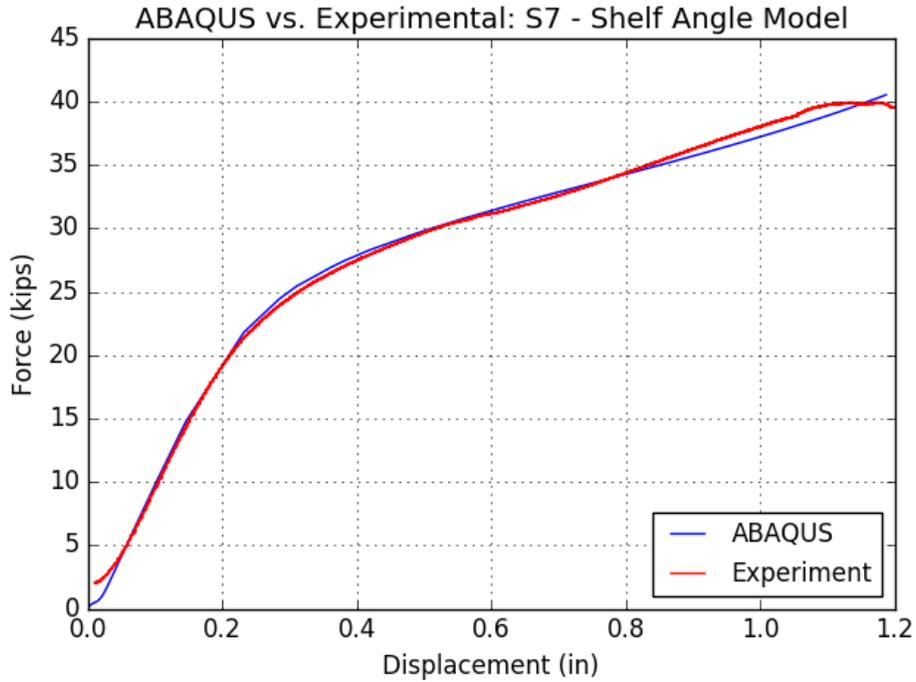
Figure 6-17 Assembly S7 – Force-Displacement, ABAQUS vs. Experimental
