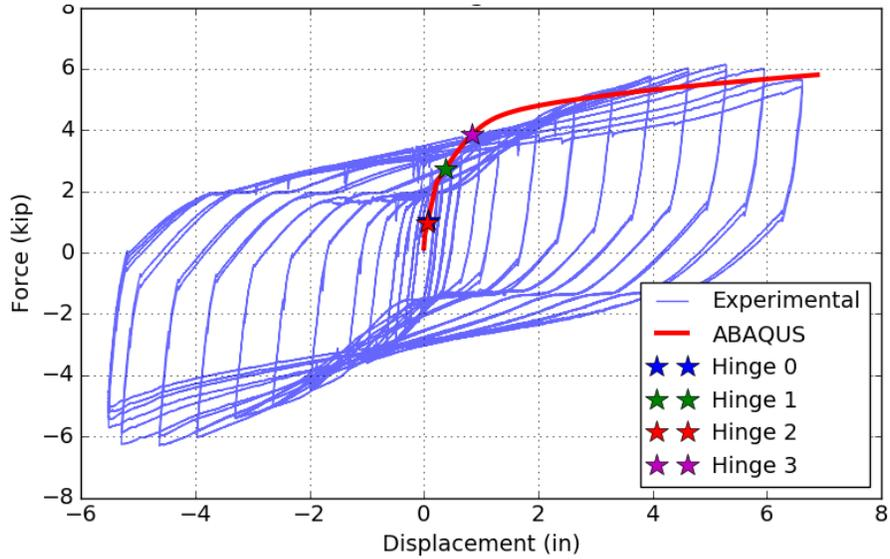
Figure 7-27: Assembly C7 – Force-Displacement, ABAQUS vs. Experimental
