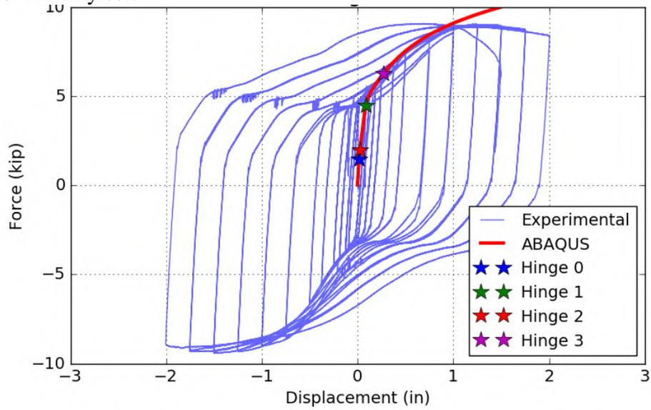
Figure 7-43: Assembly R13 – Force-Displacement, ABAQUS vs. Experimental
