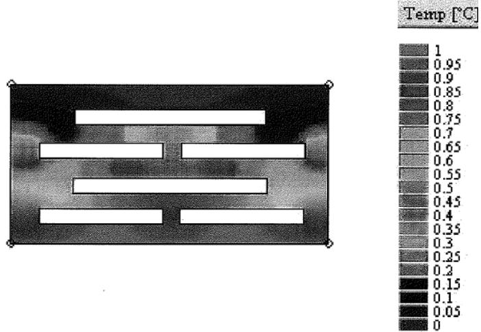
Figure 2-8: Temperature Gradient of a Slotted Channel Section
