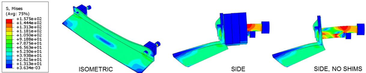
Figure 6-34 Assembly 15 – von Mises stress contour – ISO view
