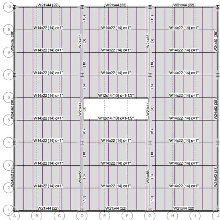
Figure 1-2: Steel framing plan as completed in RAM Steel.
