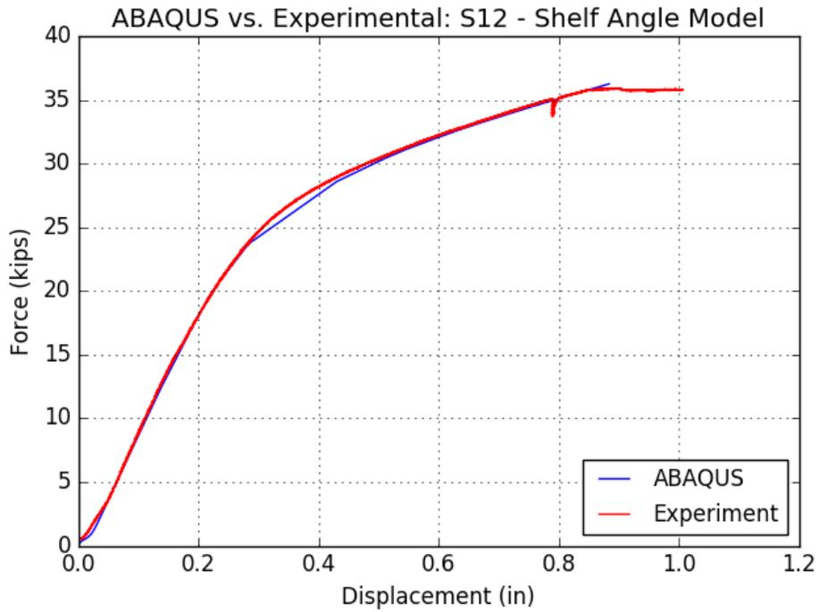
Figure 6-27 Assembly S12 – Force-Displacement, ABAQUS vs. Experimental
