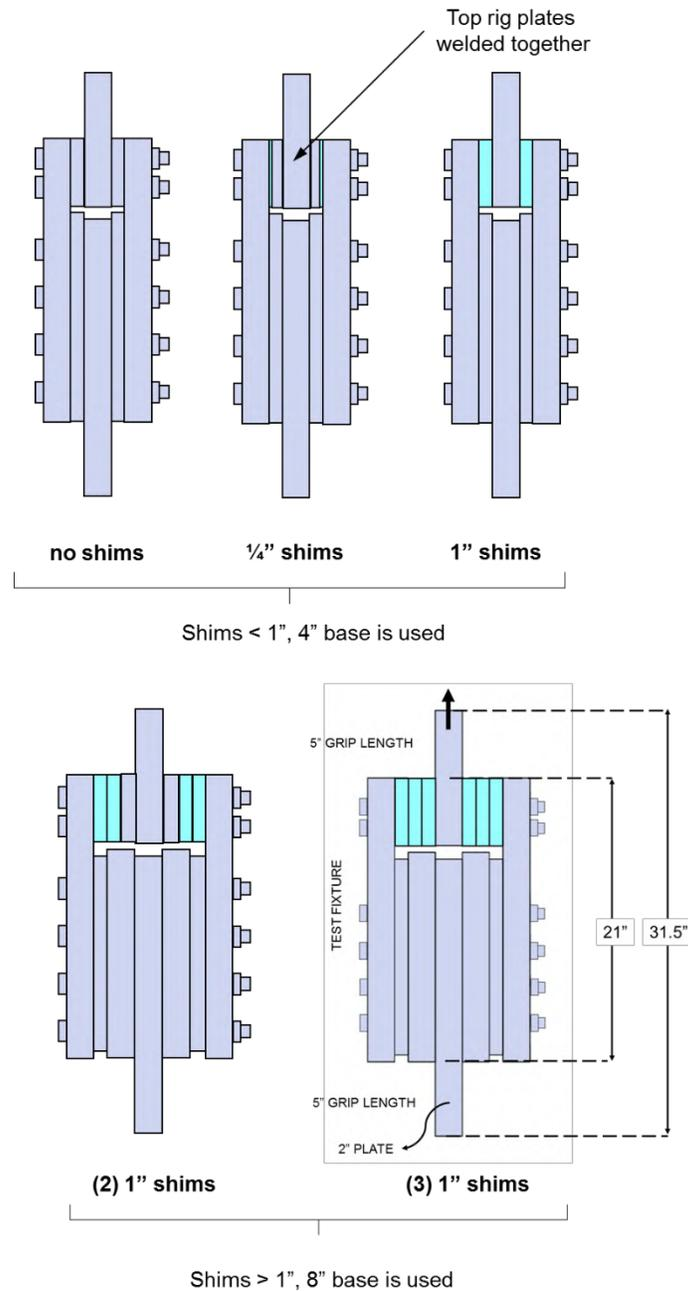
Figure 5-3: Test configuration for fills of varying thickness
