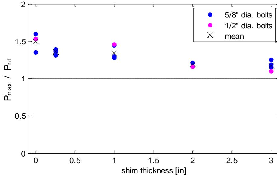
Figure 5-10: Comparison between test-to-predicted ratios per-shim thickness.
