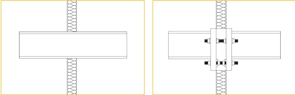
Figure 2-14: Schematic of Schoeck S22 thermal break installed in a steel canopy (Schoeck Ltd. 2015)
