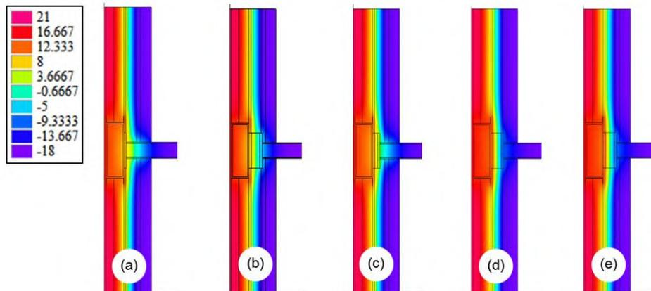
Figure 3-24: Thermal modeling of canopy beams 2D results and comparisons: a) Unmitigated, b) Vinylester shim with 3” thickness ( $\Delta\chi=8\%$ ), c) Vinylester shim with 1” thickness ( $\Delta\chi=7\%$ ), d) Proprietary 1 shim ( $\Delta\chi=30\%$ ), e) Proprietary 2 shim ( $\Delta\chi=25\%$ )
