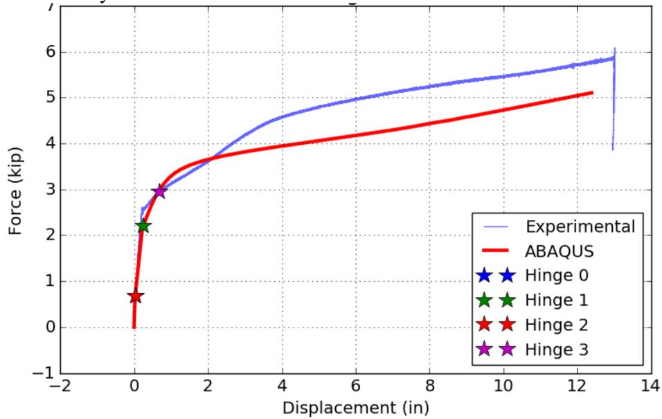
Figure 7-25: Assembly C2 – Force-Displacement, ABAQUS vs. Experimental
