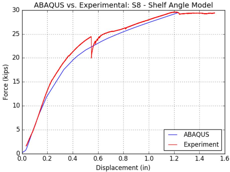
Figure 6-19 Assembly S8 – Force-Displacement, ABAQUS vs. Experimental
