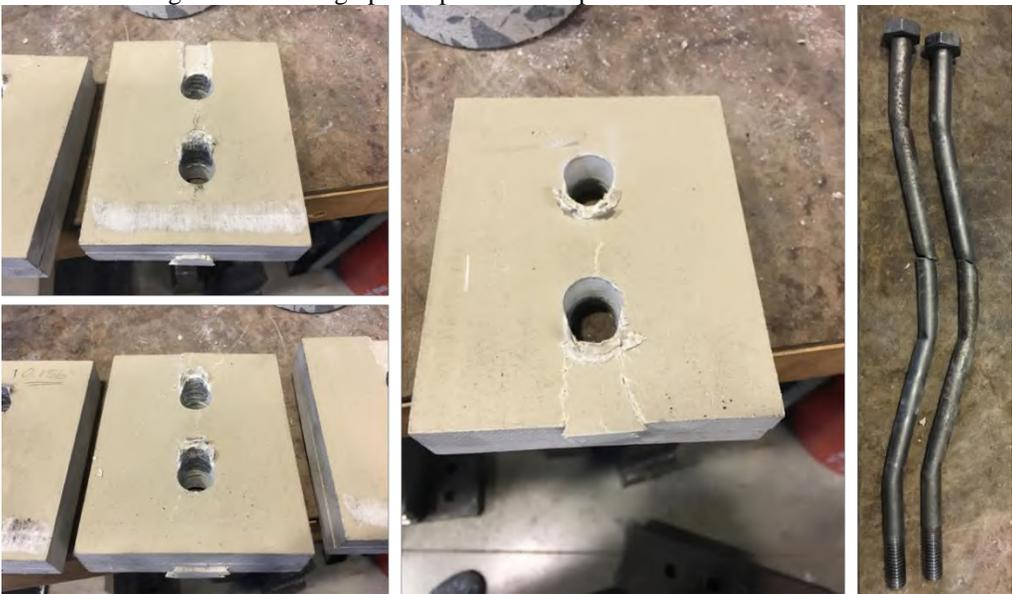
Figure 5-9: Photograph of post-failure specimens from test C16
