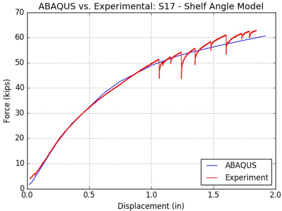
Figure 6-37 Assembly S17 – Force-Displacement, ABAQUS vs. Experimental
