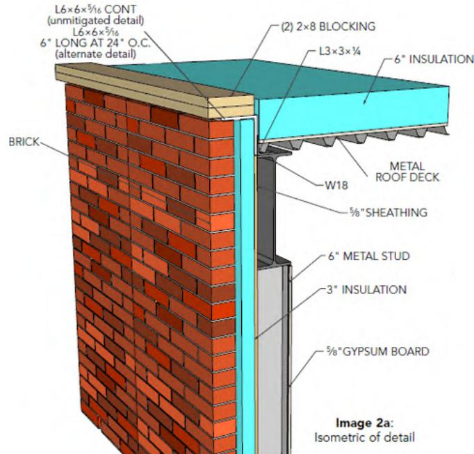
Figure 2-20: Roof Edge Angle, unmitigated (D'Aloisio, et al. 2012)
