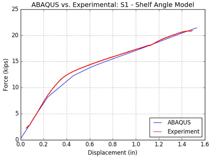
Figure 6-15 Assembly S1 – Force-Displacement, ABAQUS vs. Experimental
