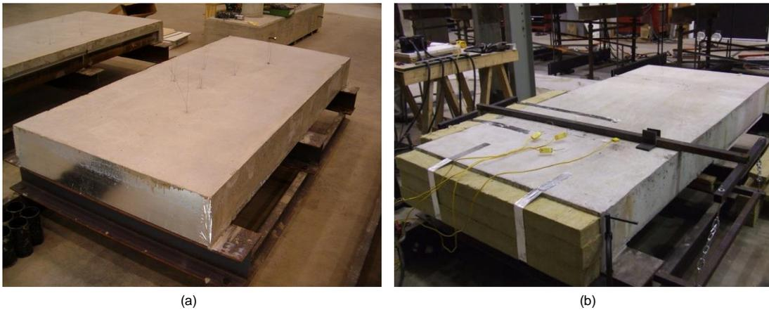
Figure 5.2: Heat transfer specimen (a) after concrete pour and (b) during testing
