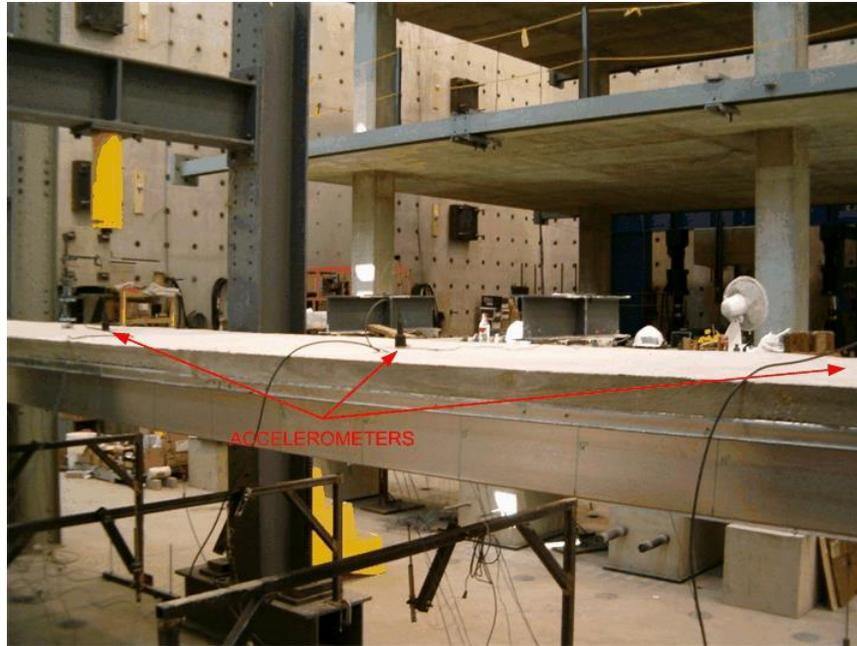
Figure 4.29: Specimen with Accelerometers Attached
