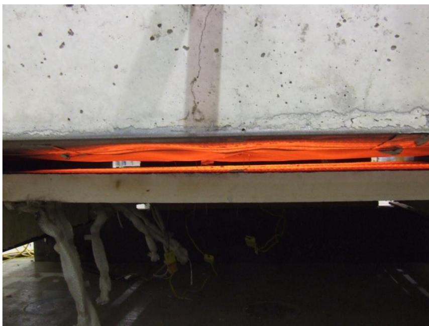
Figure 5.5: Heating of unprotected side of heat transfer specimen showing deformations of bottom plate
