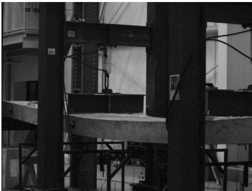
Figure 4.49: CC-DD Specimen 2 with approximately 8 in. of deflection at mid-span and 23 kips of load applied at each load point
