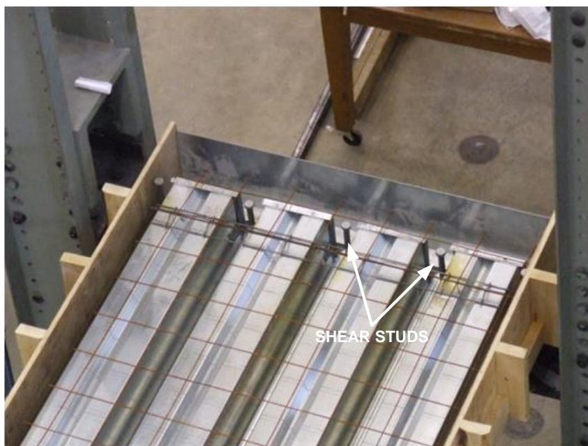
Figure 6.6: SC-DD Specimen ends before concrete casting (note shear studs at ends)
