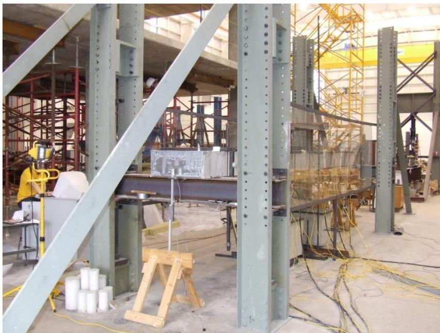
Figure 5.12: Overall view of specimen just prior to testing showing protective polycarbonate plastic
