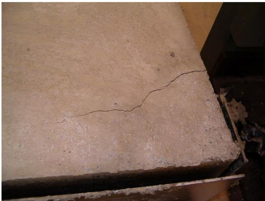
Figure 4.48: Crack the formed over north support of Specimen 2
