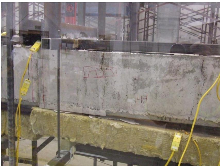
Figure 5.18: Photograph showing vertical side crack on specimen
