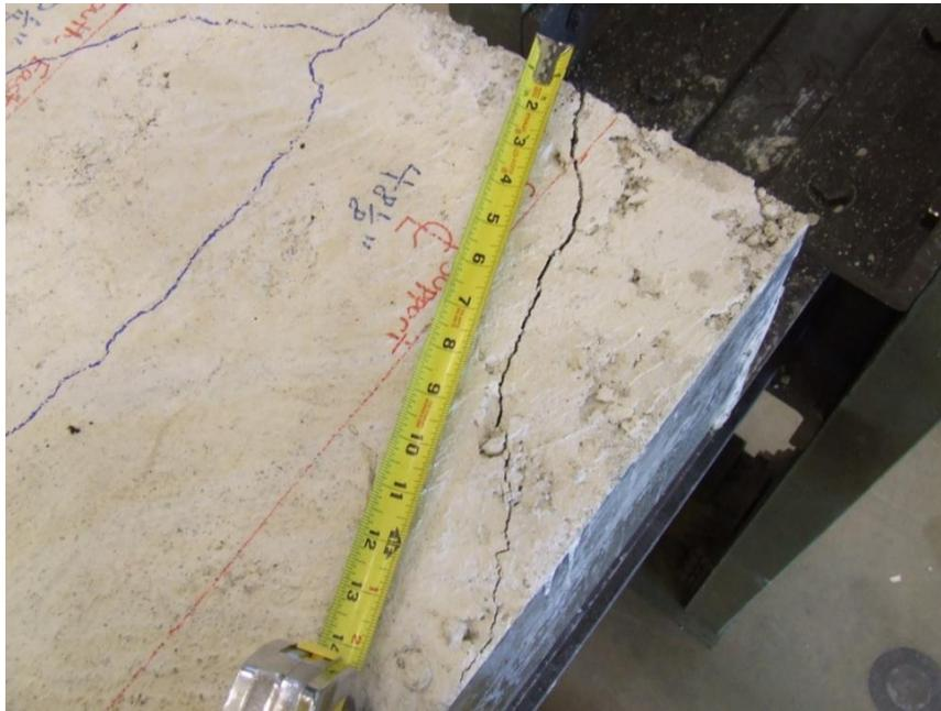
Figure 4.64: Picture of crack that formed at south support
