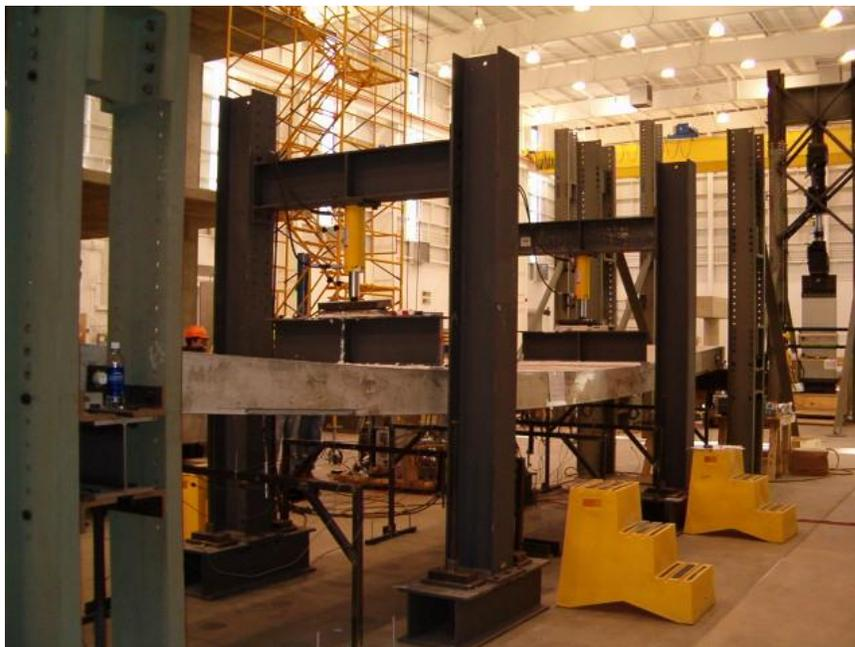
Figure 4.42: Specimen 1 with approximately 6 in. of deflection at mid-span and 23 kips of load applied at each load point (load cycle 1)
