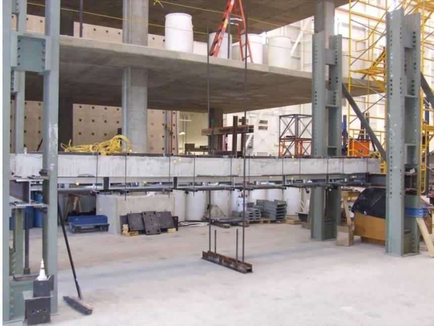
Figure 5.8: Overall Specimen view showing loading frame and heaters attached to specimen
