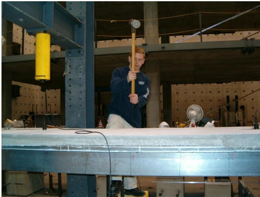
Figure 4.28: Applying Impact with Modal Hammer to test Specimen
