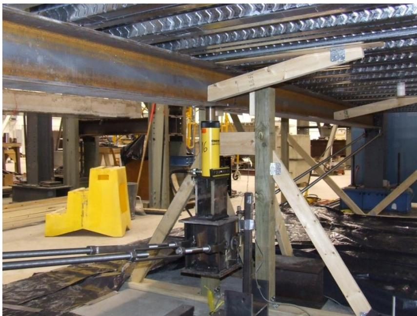
Figure 8.9: Mid-Span fixture for PLSS lab specimen
