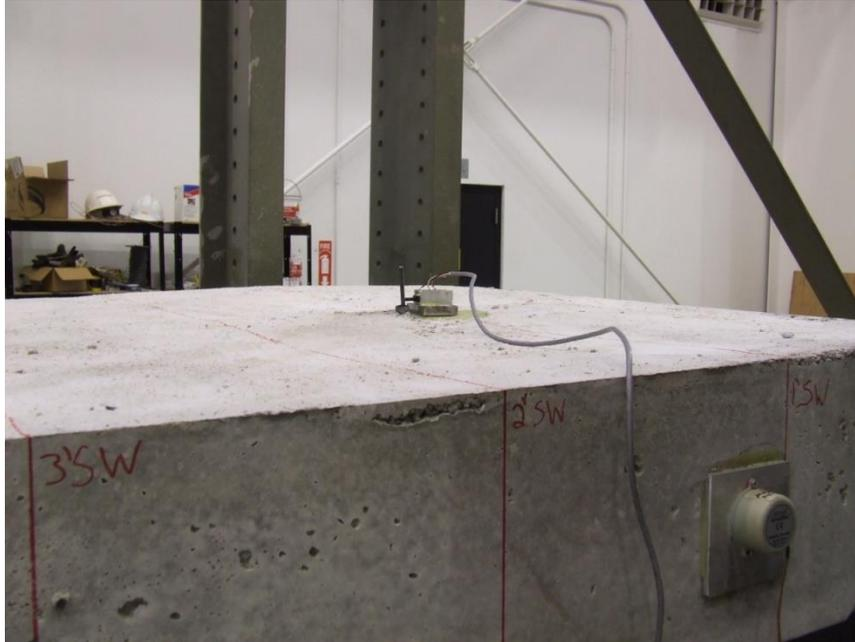
Figure 4.22: Photograph of slip sensor on CC-DD specimen
