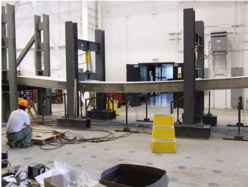
Figure 6.19: SC-DD Specimen with approximately 11 kips (220 psf) applied and 4.5 in. of deflection
