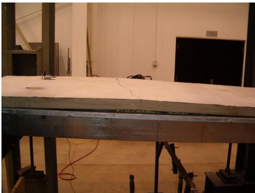
Figure 7.10: Separation of concrete from steel and concrete buckling
