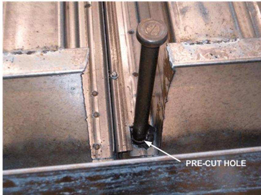
Figure 3.8: Shear Stud Placed in Test Specimen
