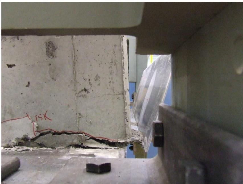
Figure 4.57: Propagation of shear bond failure to north end
