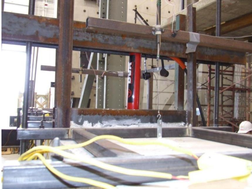
Figure 5.10: Photograph showing displacement transducer
