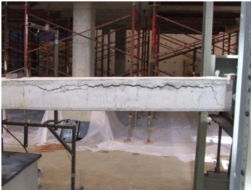
Figure 5.29: Growth of crack at north end during load test
