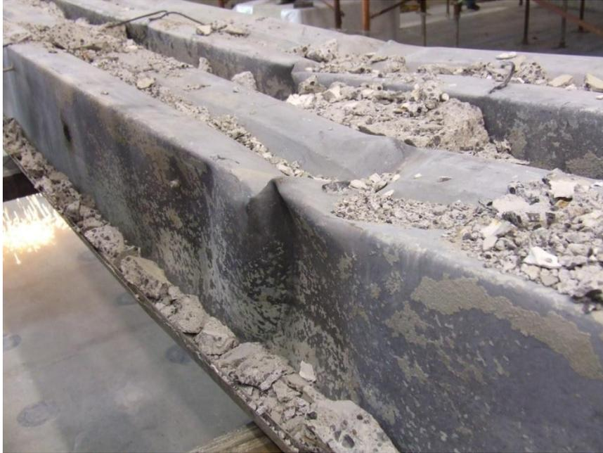
Figure 5.32: Buckled steel deck near mid-span (concrete was removed)
