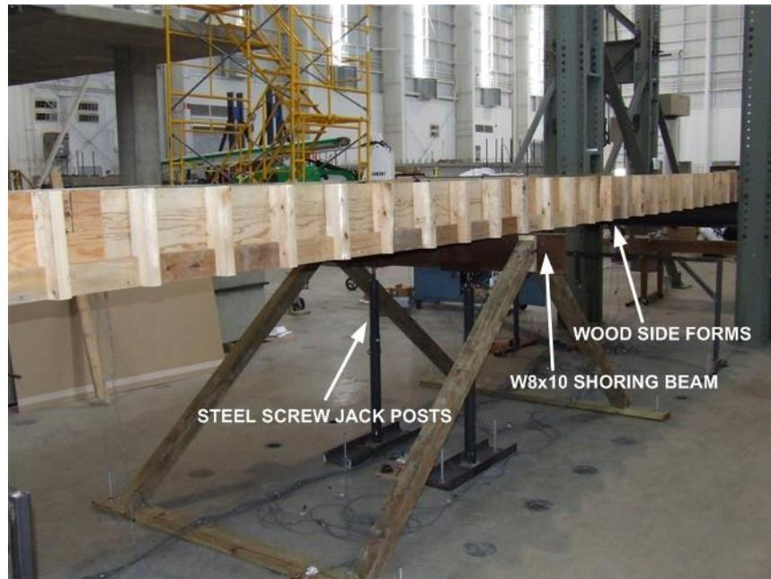
Figure 6.7: SC-DD Specimen prior to concrete casting
