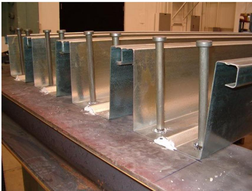
Figure 7.5: View of specimen with shear studs placed
