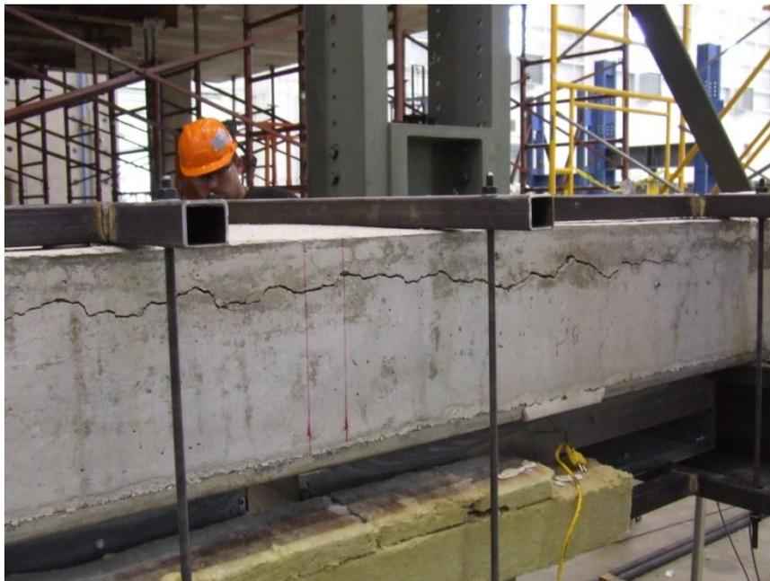
Figure 5.26: Crack that formed at north end at end of heating
