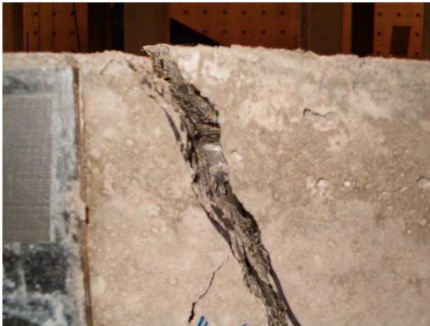
Figure 4.44: Close-up of southeast support crack during re-loading of Specimen 1
