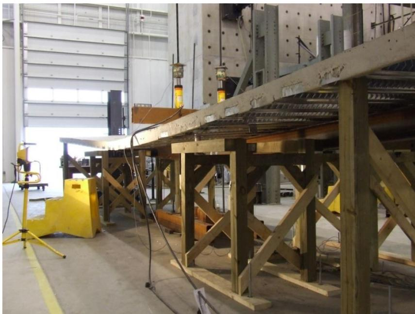
Figure 8.21: Side view of PLSS Specimen with 7.5 in. of mid-span deflection
