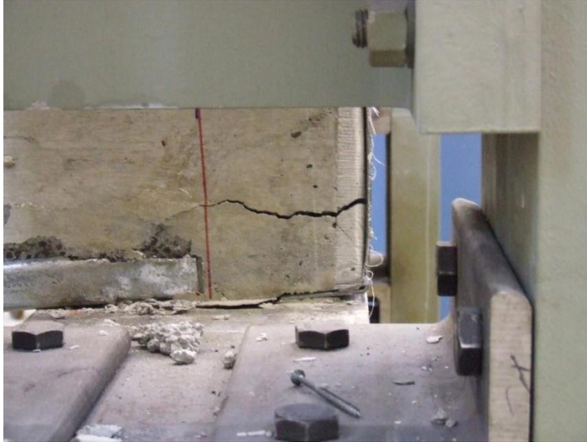
Figure 6.20: Concrete cracking at north support of SC-DD Specimen
