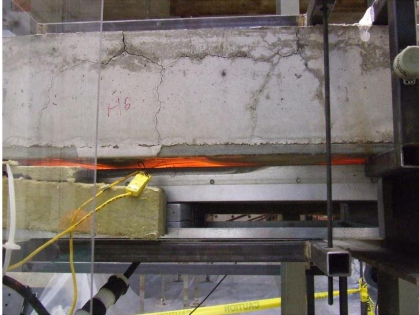
Figure 5.14: Photograph showing local upward bowing of bottom plate
