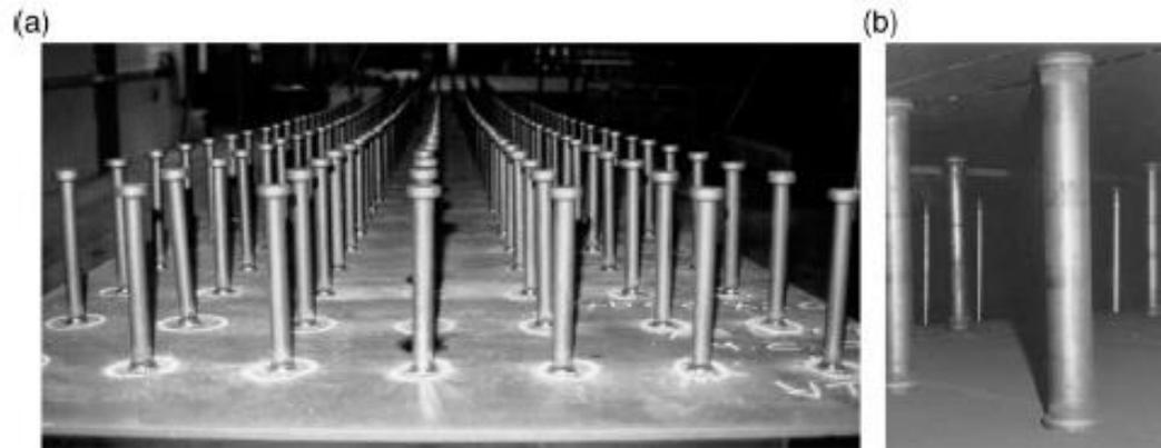
Figure 2.8: DSC with (a) traditional shear studs and (b) Bi-Steel System (McKinley & Boswell, 2002)
