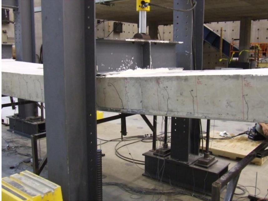
Figure 6.18: View of north load point just prior to shear bond failure
