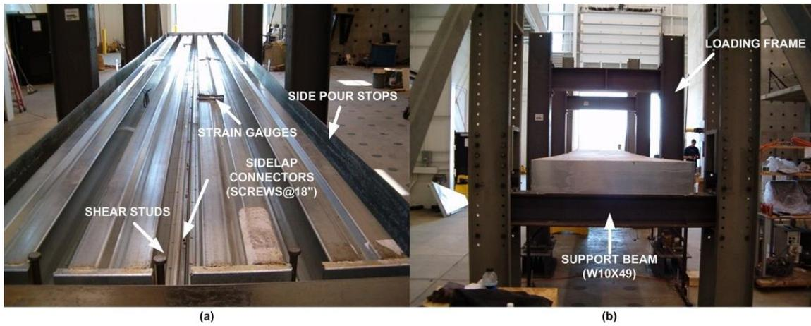
Figure 4.17: CC-DD Floor System Specimen (a) Before and (b) After Concrete Placement
