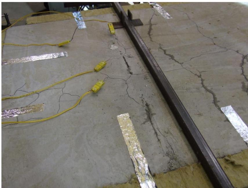
Figure 5.6: Picture of specimen showing cracks in concrete
