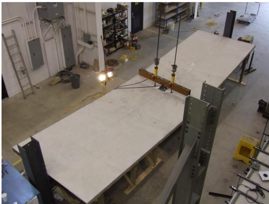
Figure 8.20: Photograph from above of PLSS Specimen at 6.5 in. of mid-span deflection
