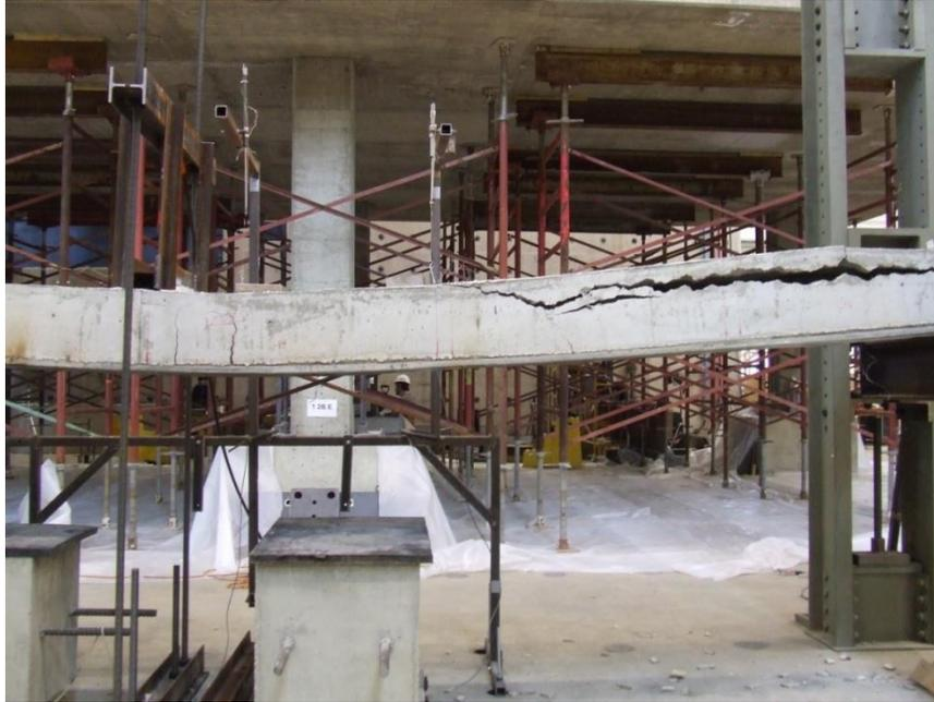
Figure 5.30: Vertical separation of slab from deck during load test
