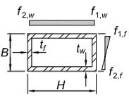
Compression and/or minor-axis bending  | N/A                                                                                                                                                                   | $\zeta = \frac{t_f}{t_w} \left( 0.53 - \frac{a_w}{\phi} \right)$ $a_w = 0.63 - 0.1 \frac{H}{B} \leq 0.53$ |
