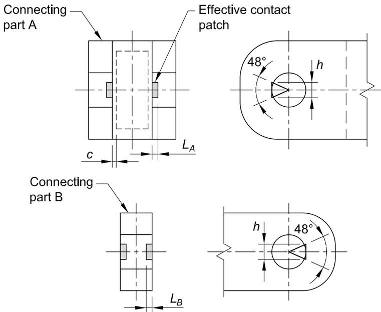
Fig. C-J8.2. Effective contact patches.
