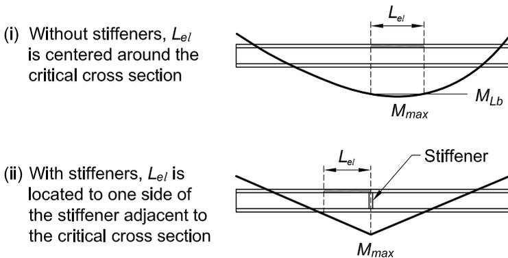
*Fig. C-A-1.1. Moment diagrams and strain averaging approach.*
