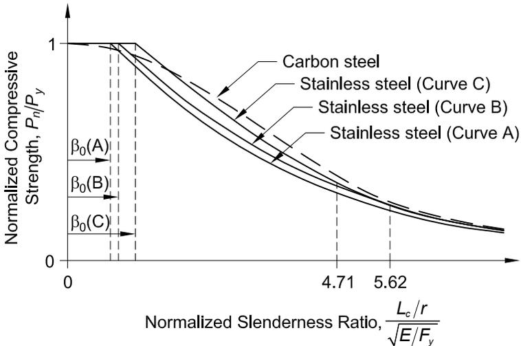
Curve A: I-shaped columns buckling about the minor axis, and other shapes
