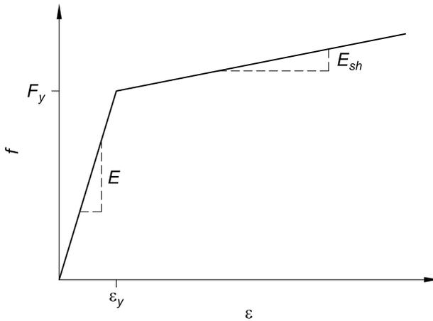
Fig. A-2.2.1. CSM material model.
