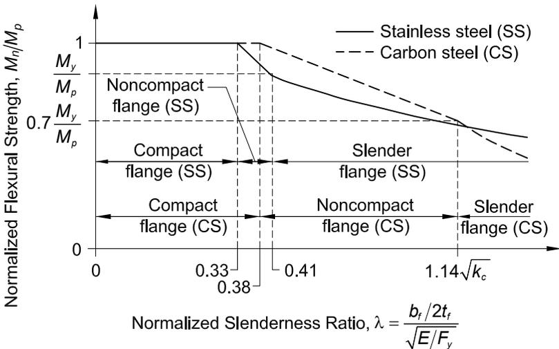
Fig. C-F1.1. Nominal flexural strength as a function of the flange width-to-thickness ratio of welded I-shapes made of stainless steel and carbon steel.
