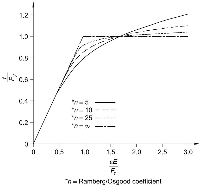
*Fig. C-A-7.1. Effect of the n coefficient on the nonlinearity of the stress-strain curve.*
