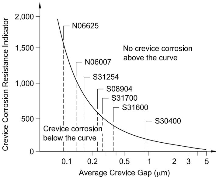
Fig. C-A3.1. Approximate corrosion resistance limits for various gap (i.e., crevice) thicknesses in ambient sea water for some common corrosion-resistant materials (ISSF, 2002).
