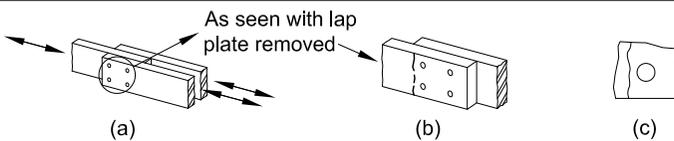
(Note: Figures are for slip-critical bolted connections.)
