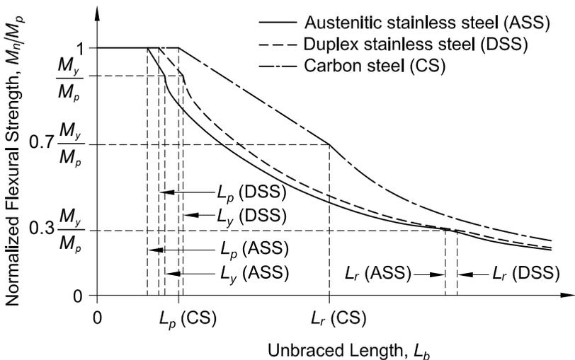
Fig. C-F1.2. Nominal flexural strength as a function of unbraced length of I-shapes made of stainless steel and carbon steel.
