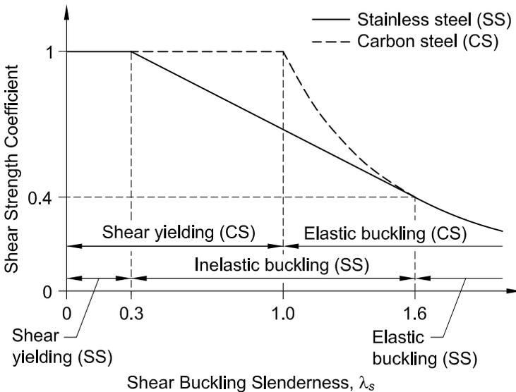
Fig. C-G4.1. Shear buckling coefficients for austenitic and duplex stainless steel, and carbon steel round HSS of medium and long lengths subject to transverse shear.
