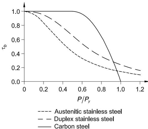
Fig. C-C2.1. Stiffness reduction factor,  $\tau_b$ , for typical austenitic and duplex grades of stainless steel for I-shaped sections buckling about the minor axis.
