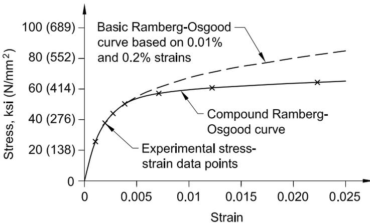
Fig. C-A-7.2. Comparison between compound and basic Ramberg-Osgood models.
