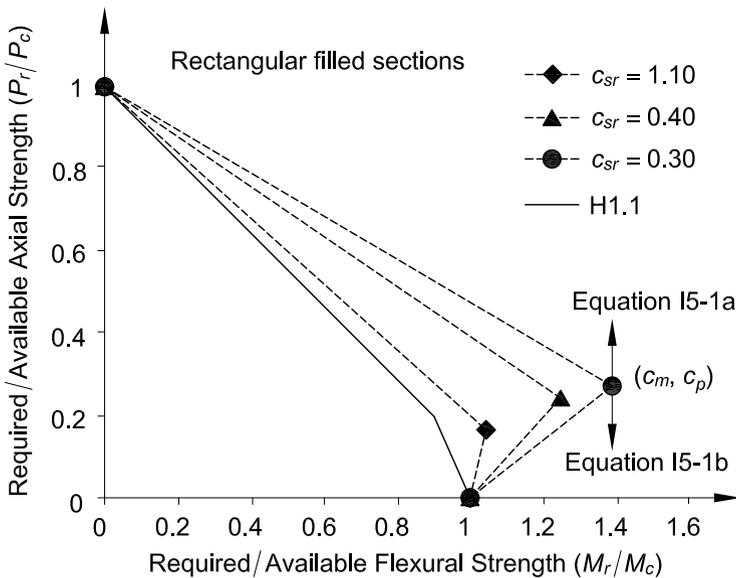
Fig. C-15.4. Interaction diagram for filled composite members with noncompact or slender cross section developed using Equations I5-1a and b.
