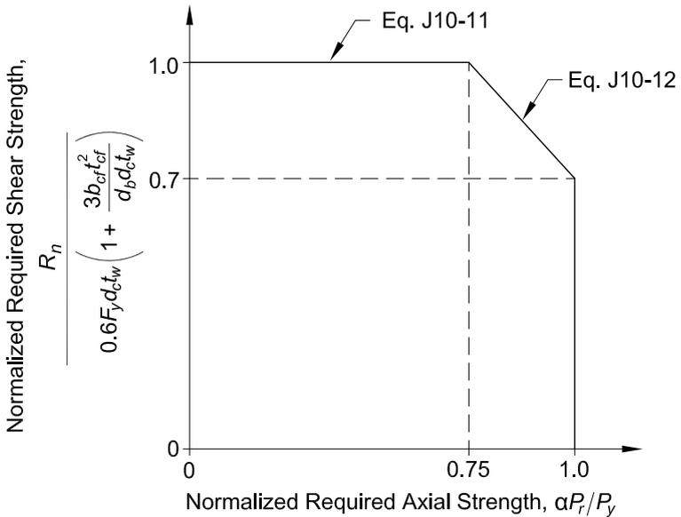
Fig. C-J10.6. Interaction of shear and axial force—inelastic.
