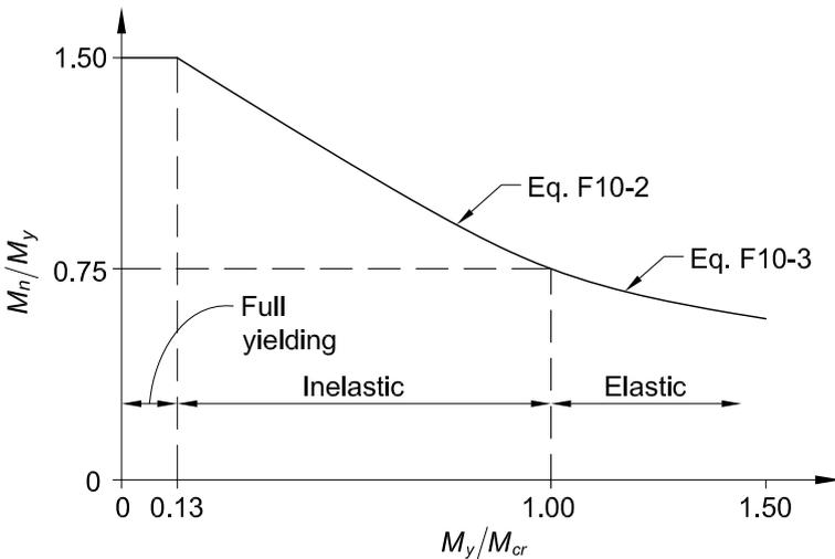
Fig. C-F10.1. Lateral-torsional buckling limits of a single-angle beam.
