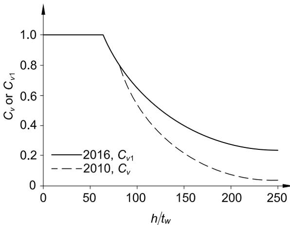
Fig. C-G2.1. Shear buckling coefficient for  $F_y = 50$  ksi (345 MPa).
