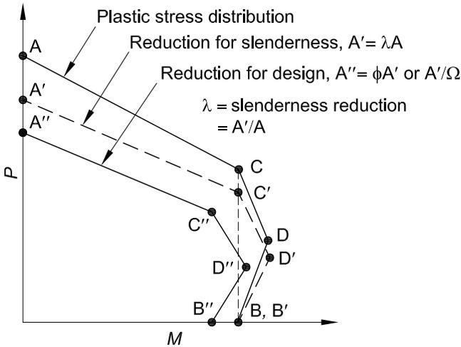
Fig. C-I5.2. Interaction diagram for composite beam-columns—Method 2.
