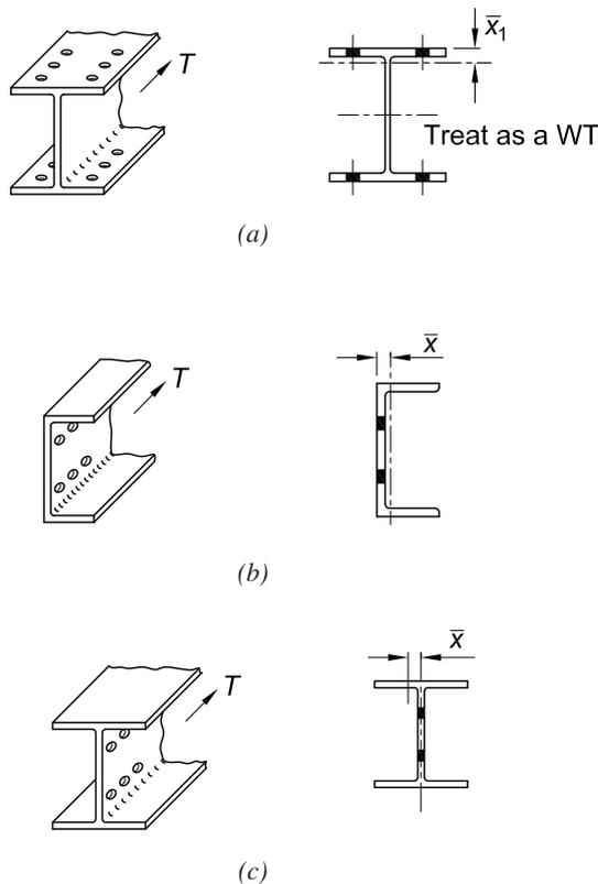
Fig. C-D3.1. Determination of  $\bar{x}$  for  $U$ .
