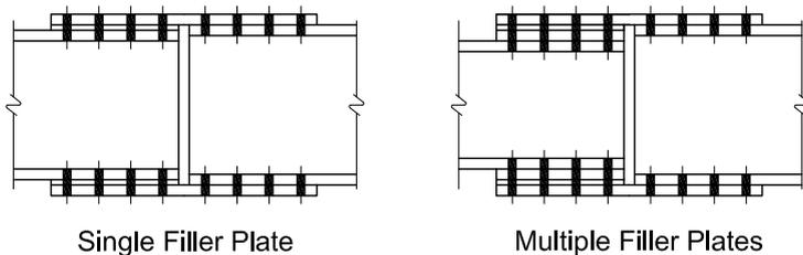
Fig C-J3.3. Single and multiple filler plate configurations.
