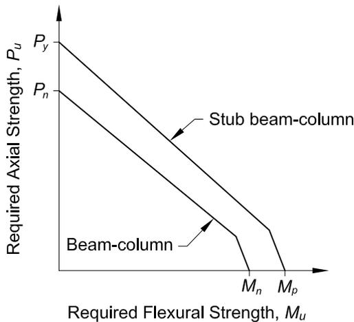
Fig. C-H1.3. Interaction curve for stub beam-column and beam-column.
