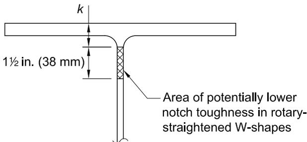
Fig. C-J10.7. Representative “k-area” of a wide-flange shape.
