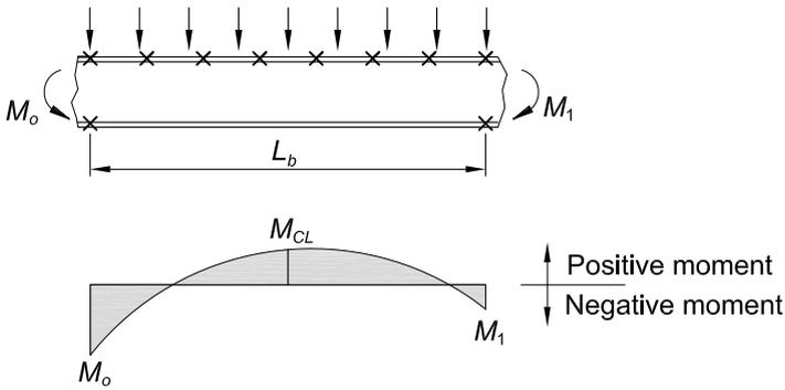
Fig. C-F1.3. Sign convention for moments in Equation C-F1-5.
