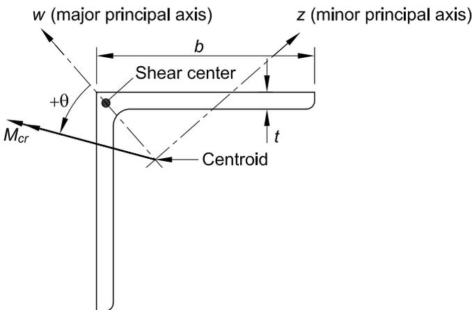
Fig. C-F10.3. Equal-leg angle with general moment loading.
