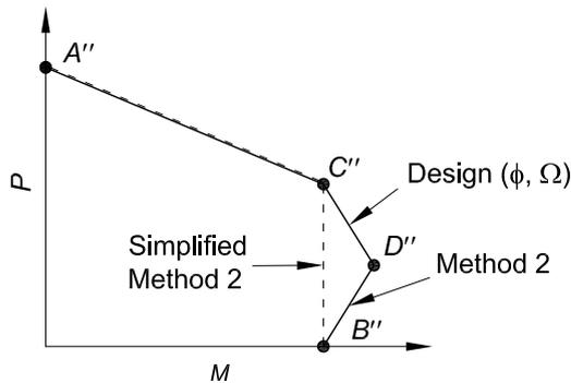
Fig. C-15.3. Interaction diagram for composite beam-columns—Method 2 simplified.
