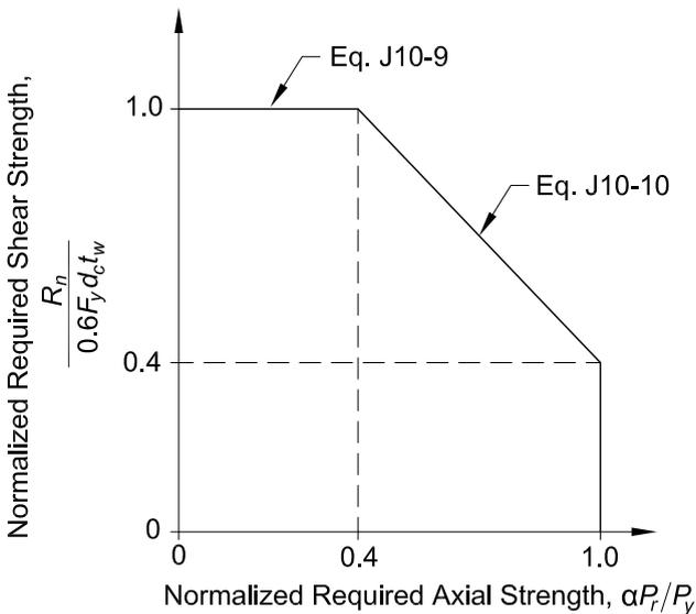
Fig. C-J10.5. Interaction of shear and axial force—elastic.
