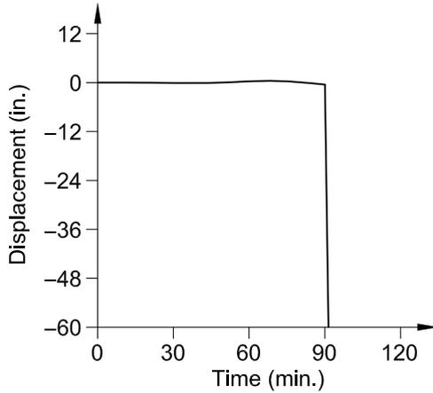
(a) Interior gravity column failure displacement history
