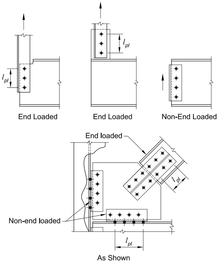
Fig. C-J3.1. End-loaded and non-end-loaded connection examples;
