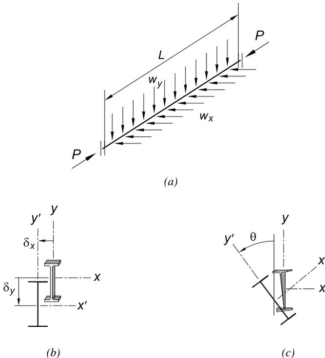
Fig. C-A-1.1. Deflection of cross section at midspan.
