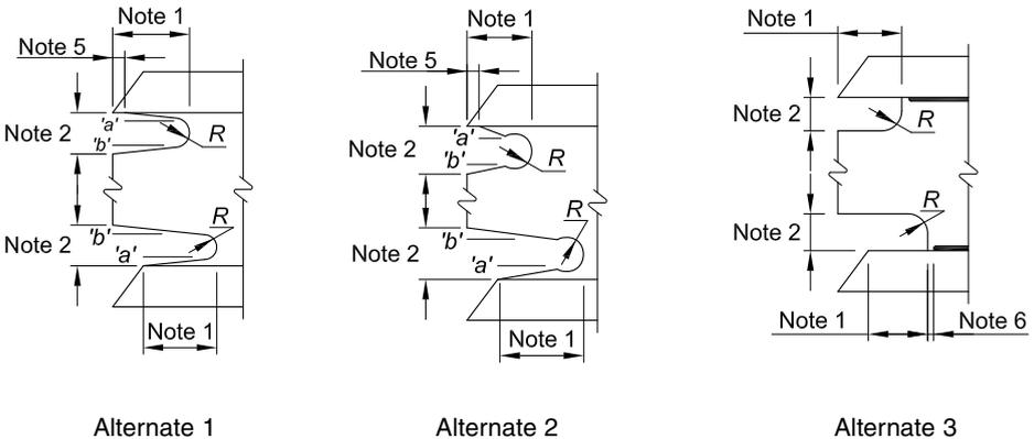
Roller shapes and built-up shapes assembled prior to cutting the weld access hole.
