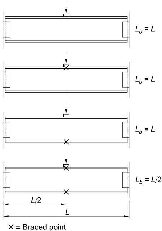
Fig. C-J10.3. Unbraced flange length for web sidesway buckling.
