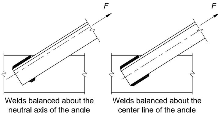
Fig. C-J1.3. Balanced welds.
