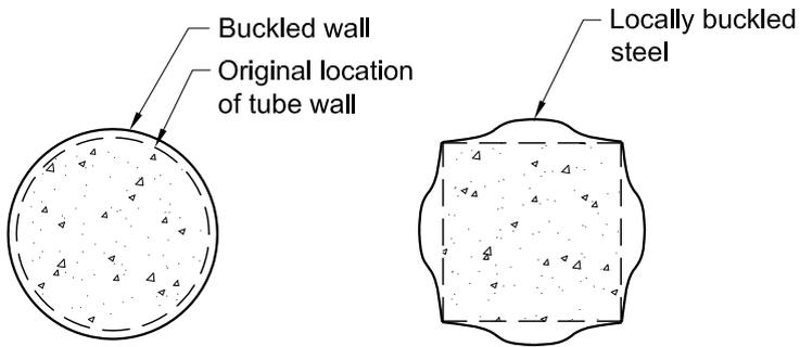
Fig. C-11.2. Cross-sectional buckling mode with concrete infill.
