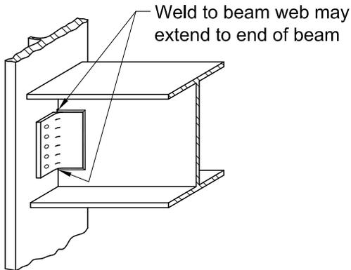
Fig. C-J2.6. Fillet weld details on framing angles.
