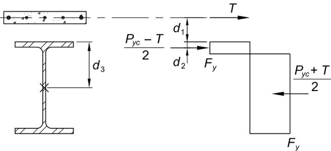
Fig. C-I3.4. Plastic stress distribution for negative moment.
