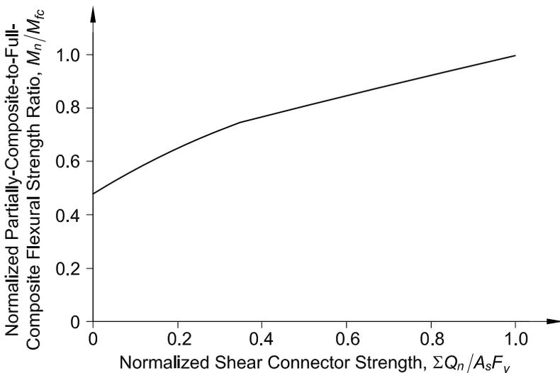
Fig. C-18.2. Normalized flexural strength versus shear connection strength ratio
