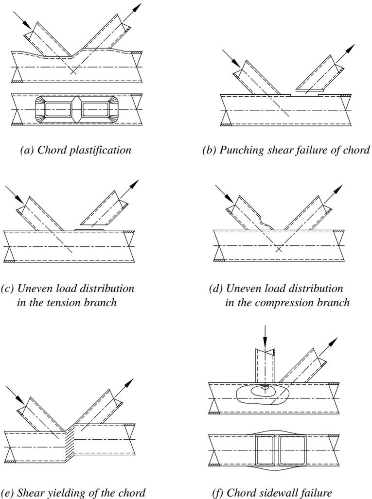
Fig. C-K3.1. Typical limit states for HSS-to-HSS truss connections.
