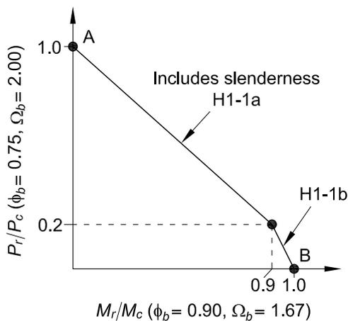
Fig. C-I5.1. Interaction diagram for composite beam-column design—Method 1.
