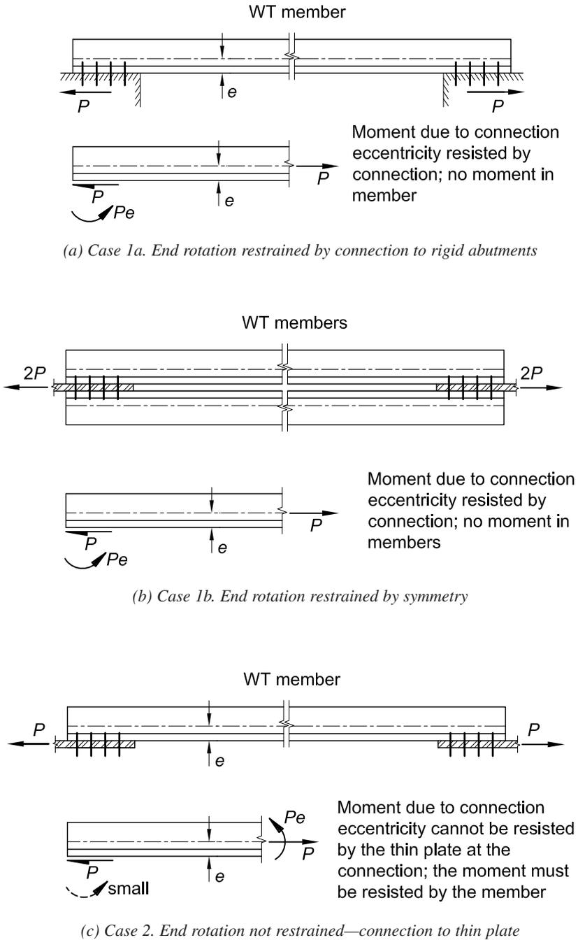
Fig. C-D3.3. The effect of connection restraint on eccentricity.
