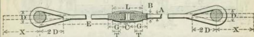
Additional length of bar beyond center of pin required to make eye for square or round bars.
