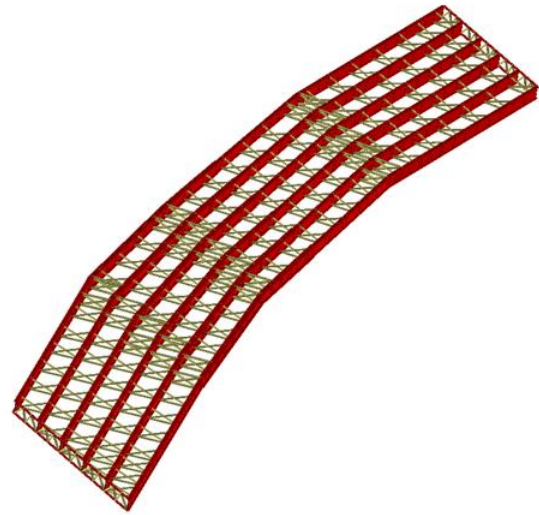
Figure 19: 3D Finite Element Model, deck removed for clarity.
